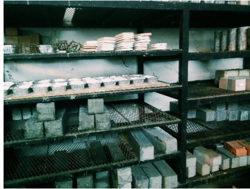
Figure 3.6 All the specimens for air curing would place at rack
