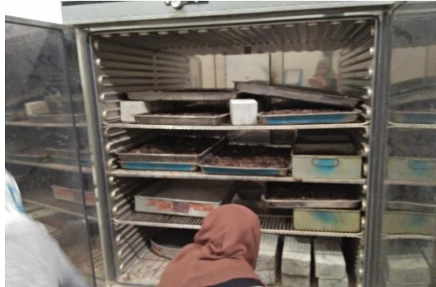
Figure 3.10 oven-dry process on brick
