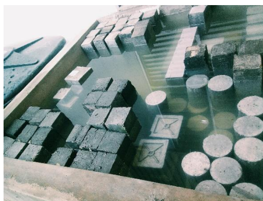
Figure 3.7 All the specimens for water curing will place at curing tank
