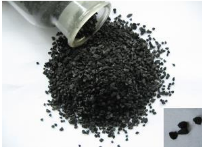
Figure 2.25: Granular Activated Carbon
