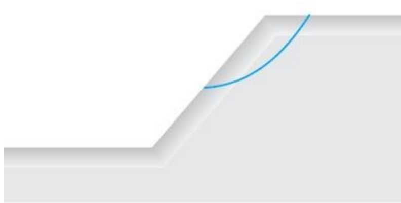
Figure 2.10 Shallow slope failure
