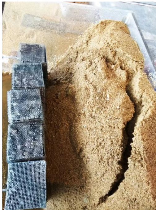
Figure 4.19 Plan view of condition of the soil slope after subjected to rainfall.
