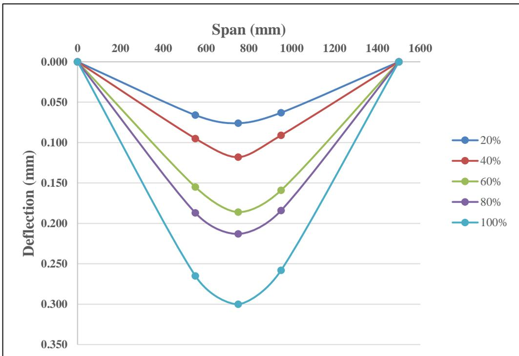
Figure 4.7 Deflection Profile for Beam 2
