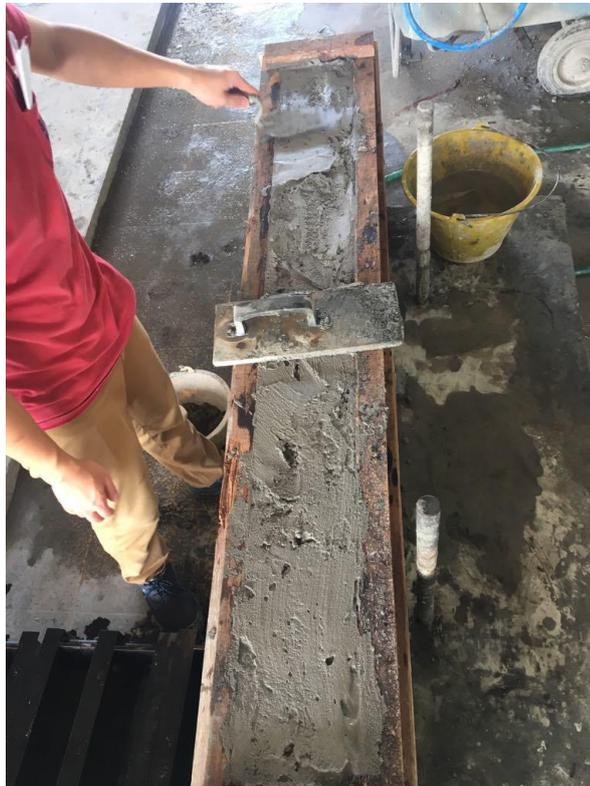
Figure 3.8 Casting of the Specimen
