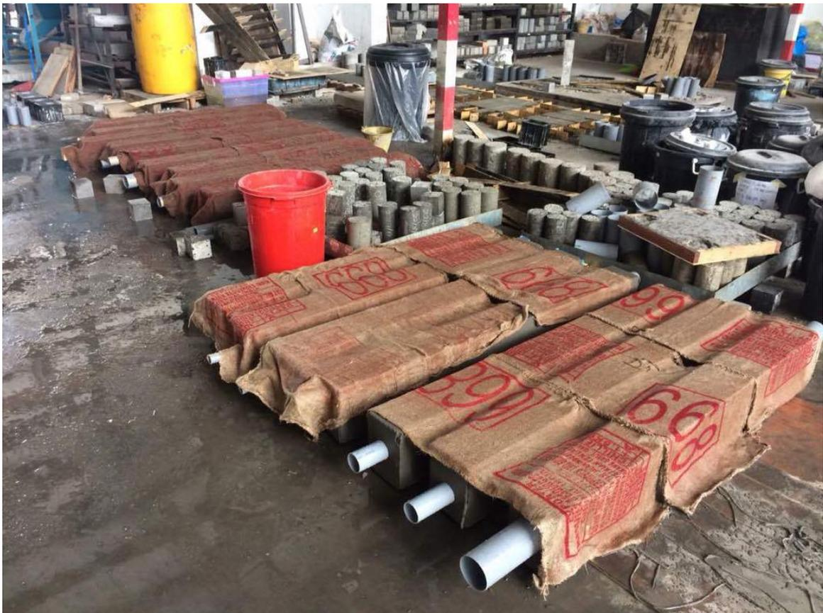
Figure 3.9 Curing Process
