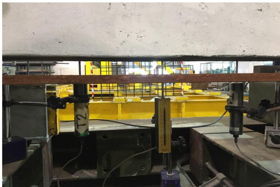
Figure 3.12 Position of LVDT
