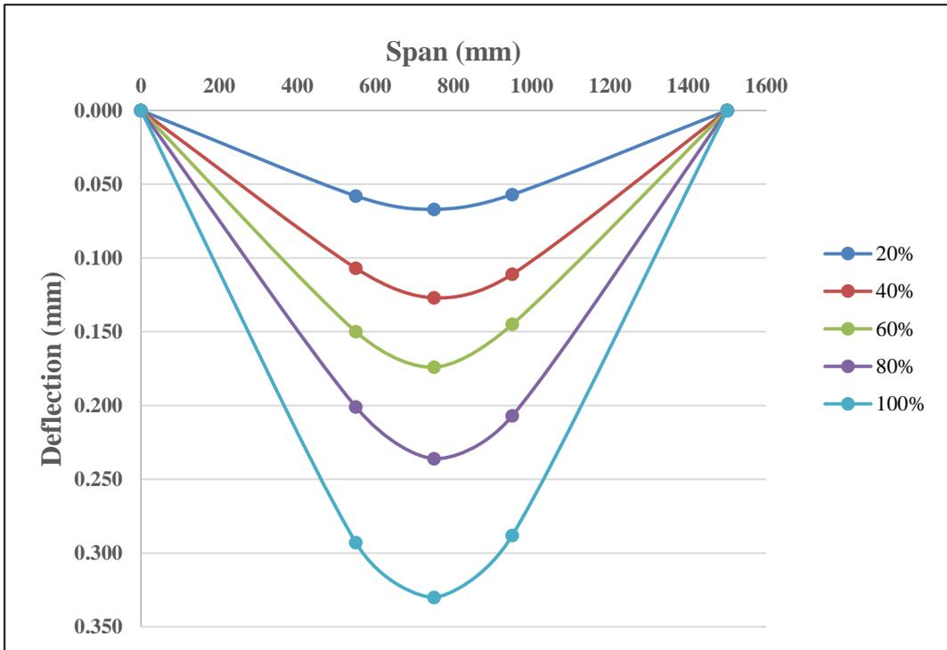
Figure 4.6 Deflection Profile for Beam 1
