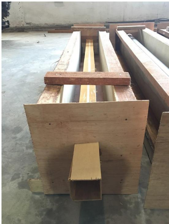
Figure 3.3 Square Hollow Section Formwork
