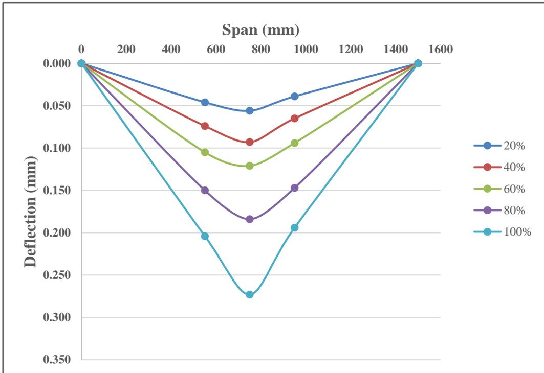
Figure 4.8 Deflection Profile for Beam 3
