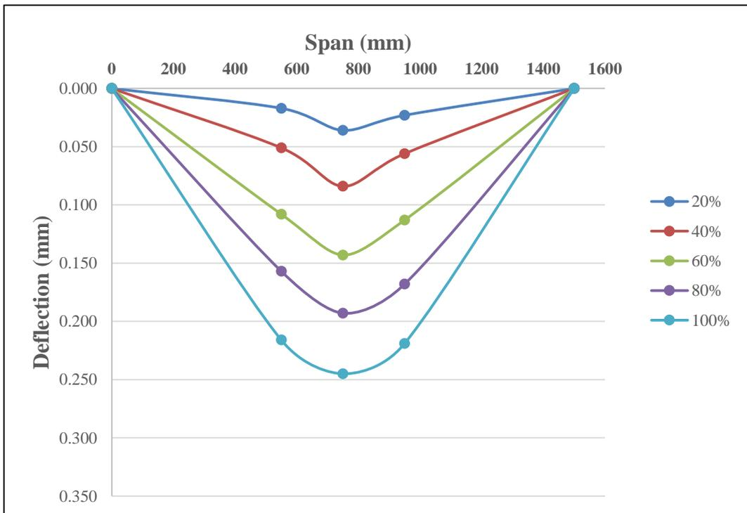
Figure 4.9 Deflection Profile for Beam 4
