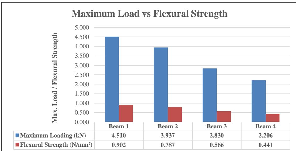
Figure 4.1 Maximum Loading and Flexural Strength of Beams
