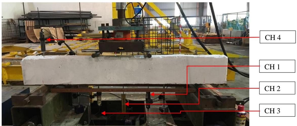
Figure 3.11 Testing Set Up of the Beam
