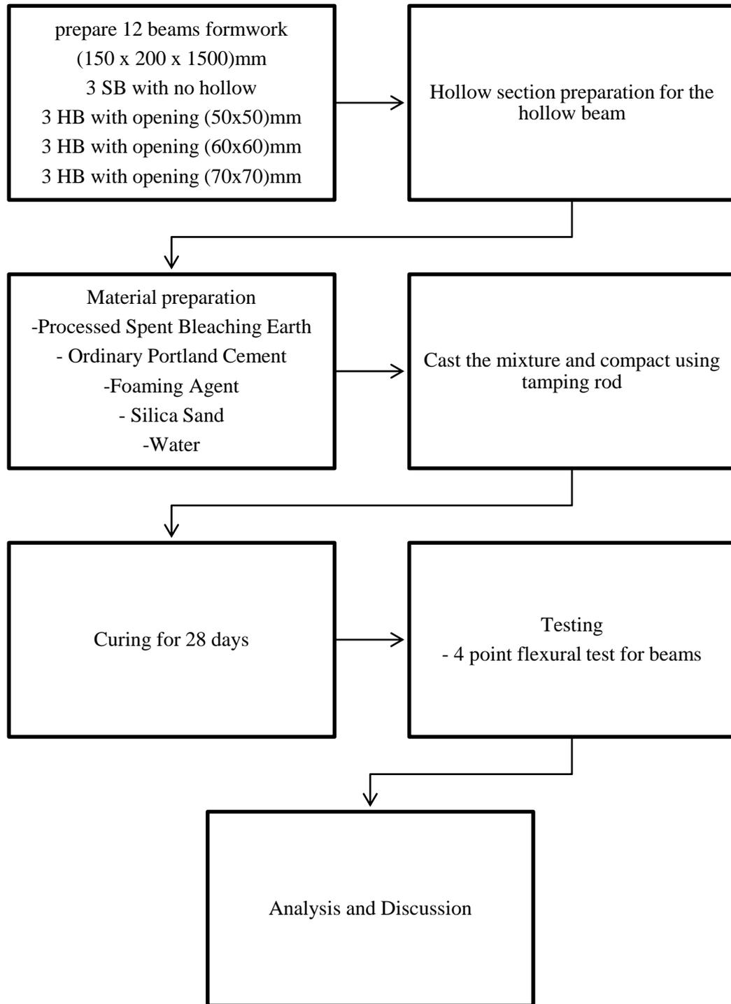
Figure 3.1 Research Experimental Works Flow
