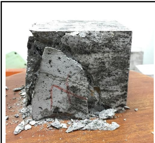
Figure 4.11 Compressive strength failure of 30% of fly ash
