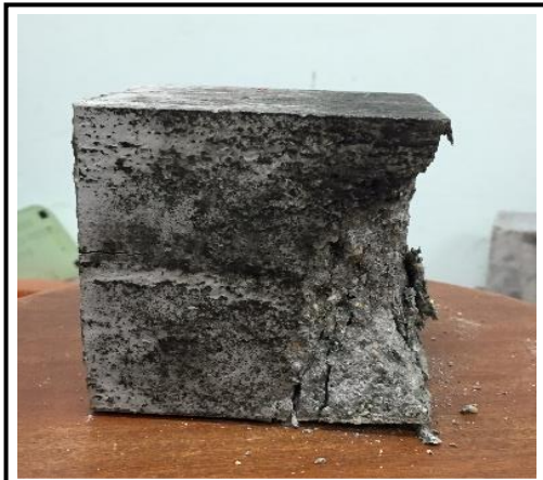
Figure 4.9 Compressive strength failure of 0% of fly ash
