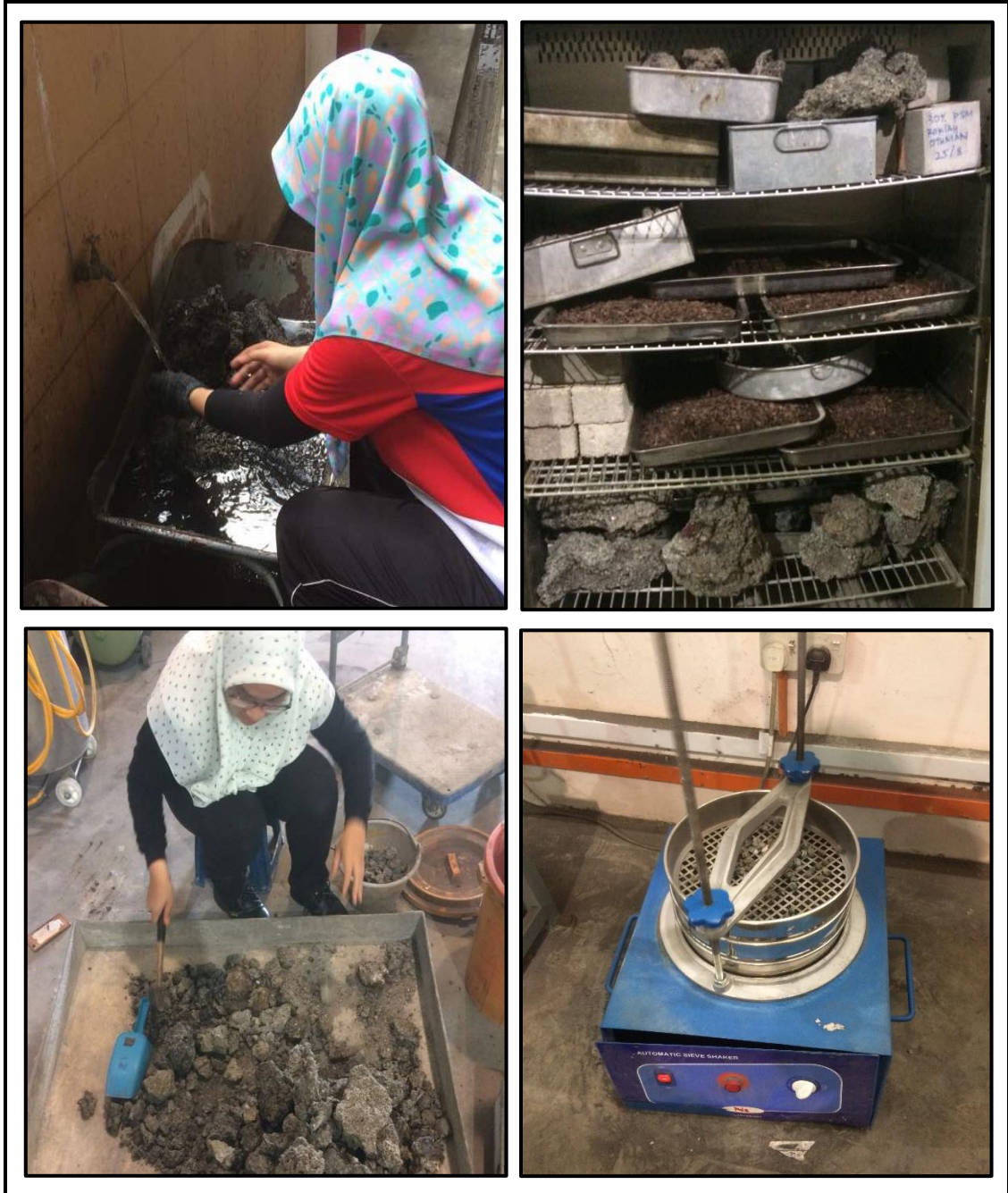
Figure 3.5 Processing of palm oil boiler stone to be lightweight aggregate.
