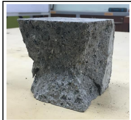
Figure 4.12 Compressive strength failure of 40% of fly ash
