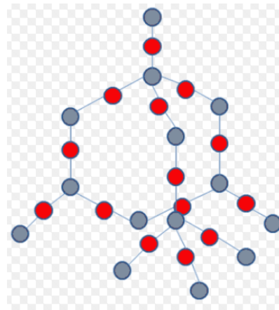
Figure 2. 4: Tetrahedron Shape of Silica
