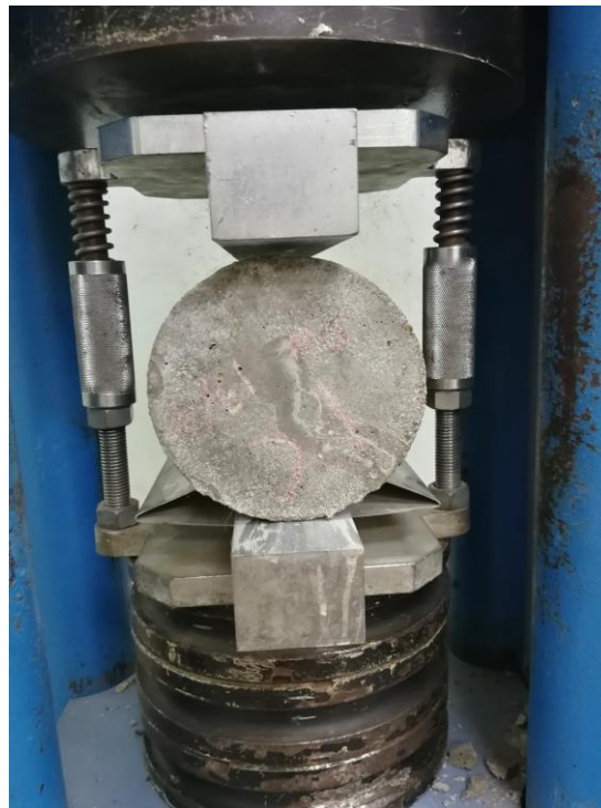
Figure 3. 10 Cylinder Samples placed into the Splitting Mould for Tensile Strength Test
