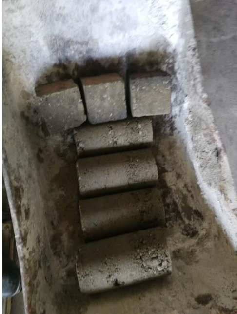
Figure 3. 5 : The samples are left for one day in the mould and move to curing tank
