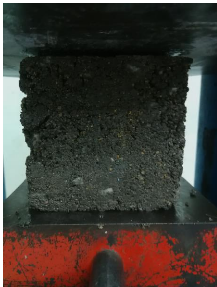
Figure 3. 9 : Cube Samples placed into the Machine for Compressive Strength Test
