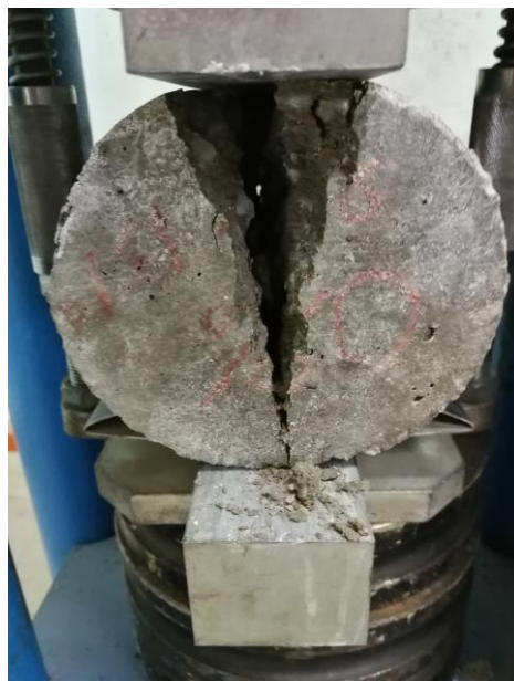
Figure 4. 4 : Pattern of the cylinder samples after tensile splitting test
