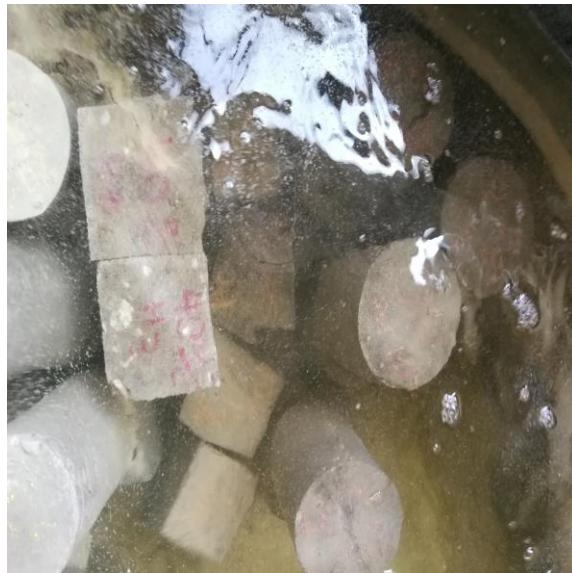
Figure 3. 6 : The samples were placed in the curing tank until the day for tested
