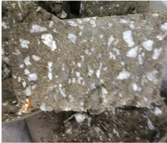
Figure 4. 5 : Structure of the 30% Samples after Tensile Splitting Test
