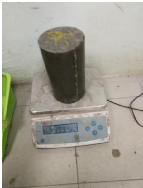
Figure 3. 7 : Samples were dried before determine its weight
