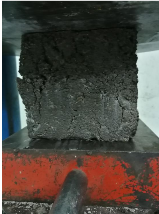
Figure 4. 2 : The pattern of the samples after compressive test
