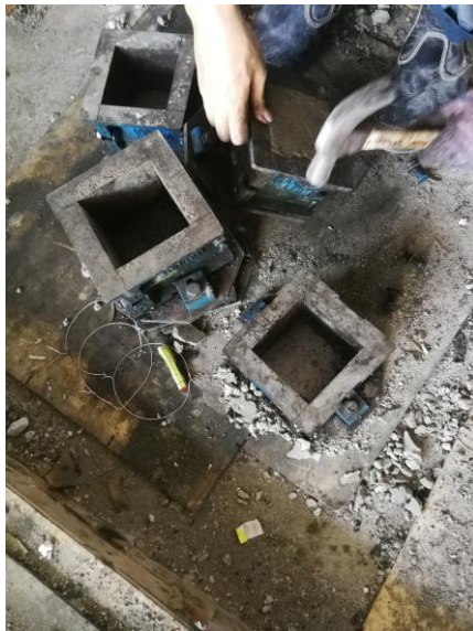
Figure 3. 4 : Prepare the mould for cube samples
