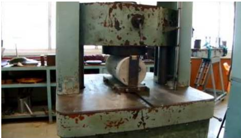
Figure 2. 7: Position of Specimen for Tensile Splitting Test
