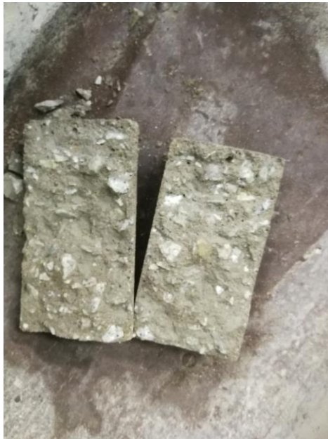
Figure 4. 6 : Structure of 0% Samples after Tensile Splitting Test
