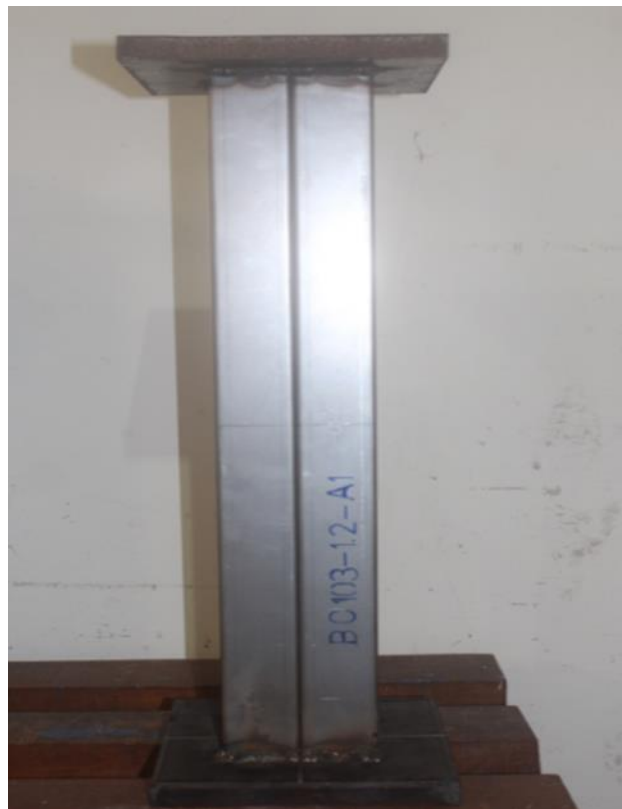
Figure 3.2 The cold-formed steel built-up I-sections
