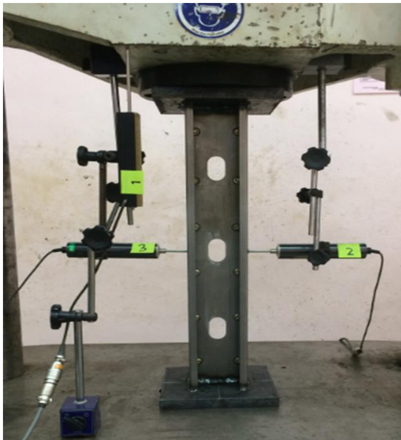
Figure 3.10 Position of the transducers
