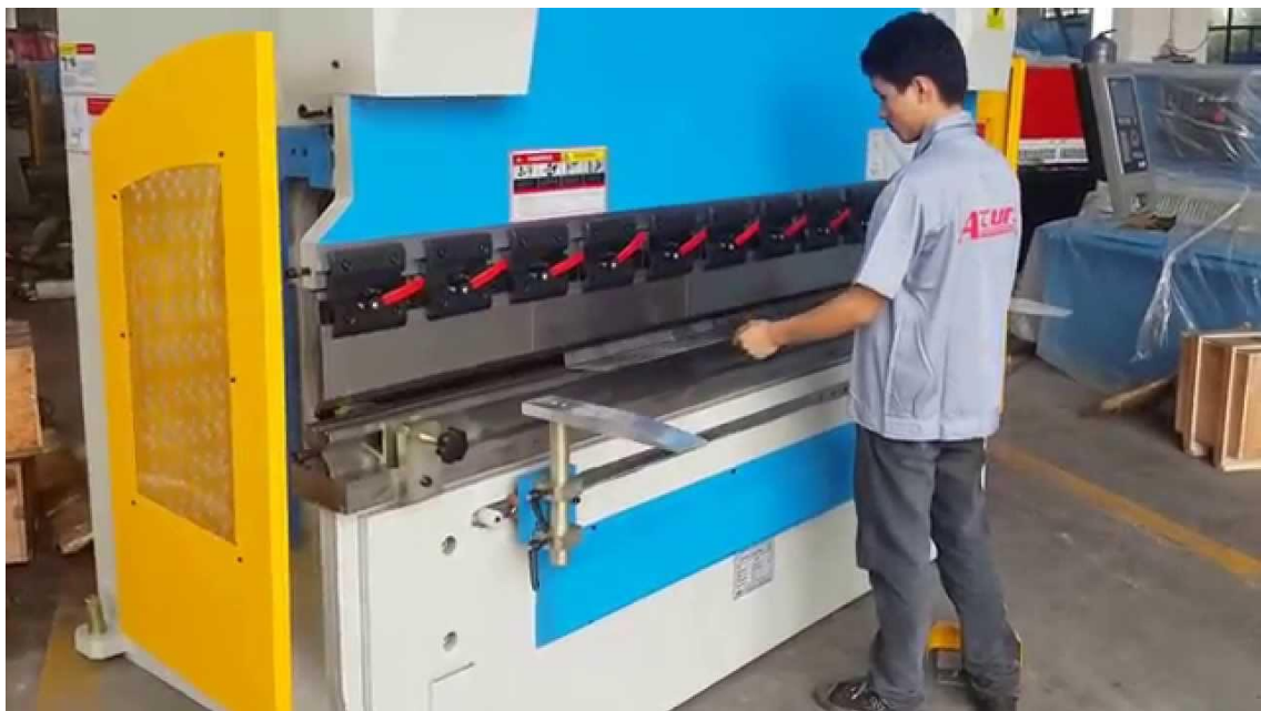
Figure 2.1 Machine use in the press breaking process Source: ANHUI LAIFU NC Machine Tool CO.LTD (2014).
