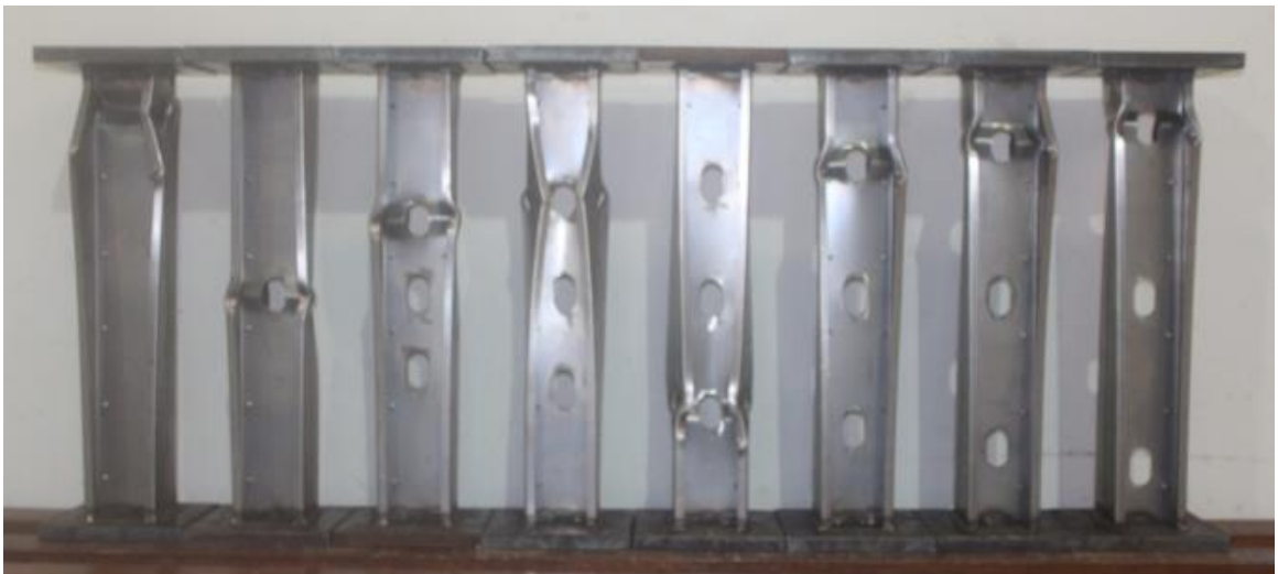
Figure 4.26 Condition of specimens from back view
