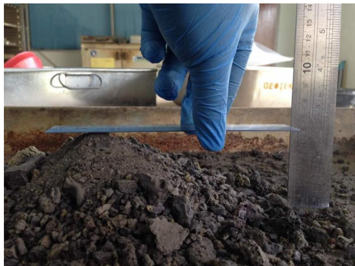
Figure 3.4: Repose angle of bottom ash
