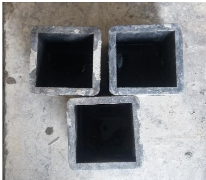
Figure 3.8 Cube mould (150 mm X 150 mm X 150 mm)
