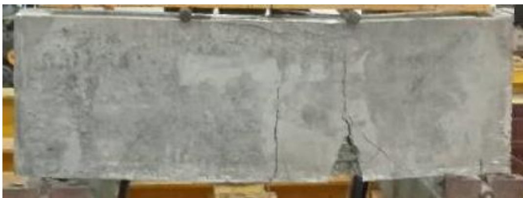
Figure 4.8 Control beam without opening
