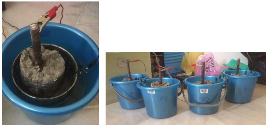
Figure 3-11 Set-up for accelerated corrosion test
