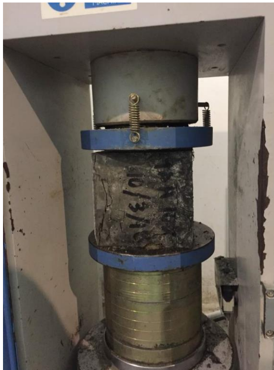
Figure 3-10 The compression testing machine
