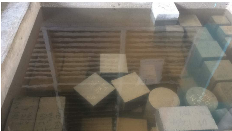
Figure 3-9 The curing tank
