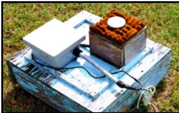
Figure 2.13 Disdrometer at Everglades National Park Source: NOAA (1999)
