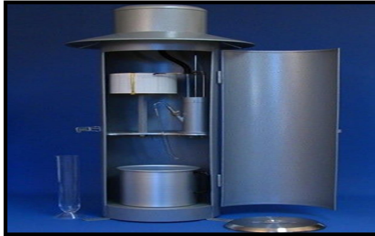
Figure 2.11 Natural syphon type rain gauge
