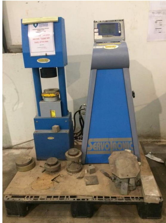
Figure 3.11: Compressive testing machine
