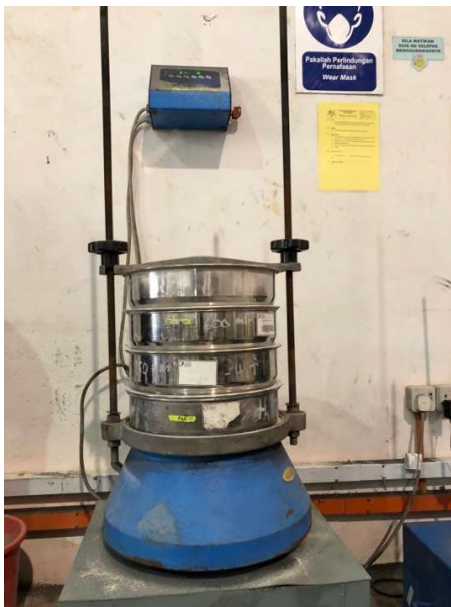
Figure 3.9: Shaker machine used to sieve sand
