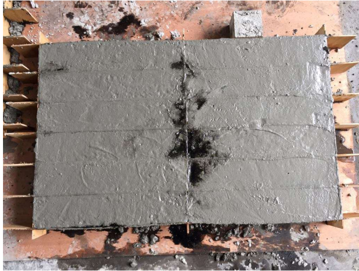
Figure 3.12: Concrete beams with size of 100mm x 100mm x 500mm
