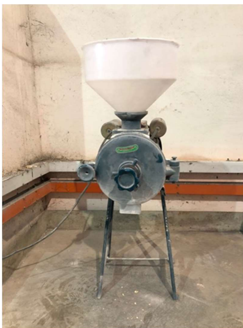
Figure 3.4: Grinding machine used for grinding eggshell
