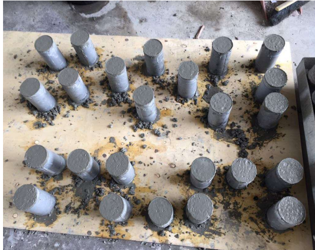
Figure 3.14: Cylinder specimen with size of 110mm diameter x 200mm height
