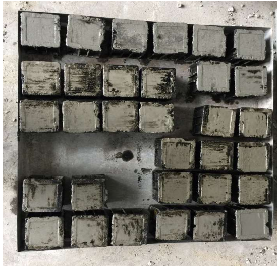
Figure 3.10: Concrete cubes with size of 100mm x100mm x 100mm
