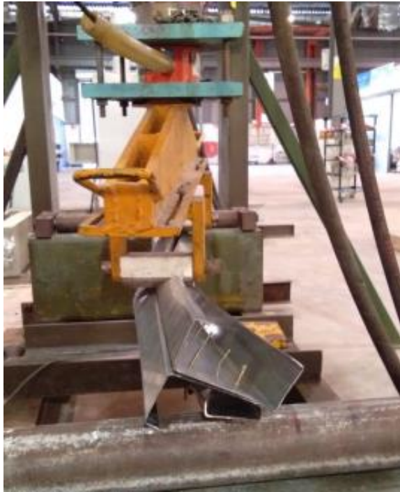
Figure 4.11 Distortional buckling occur at peak of the experiment
