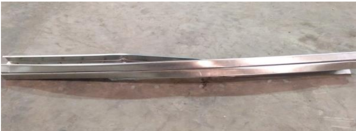
Figure 4.10 Flexural torsional buckling along the beam after experiment (post – peak)
