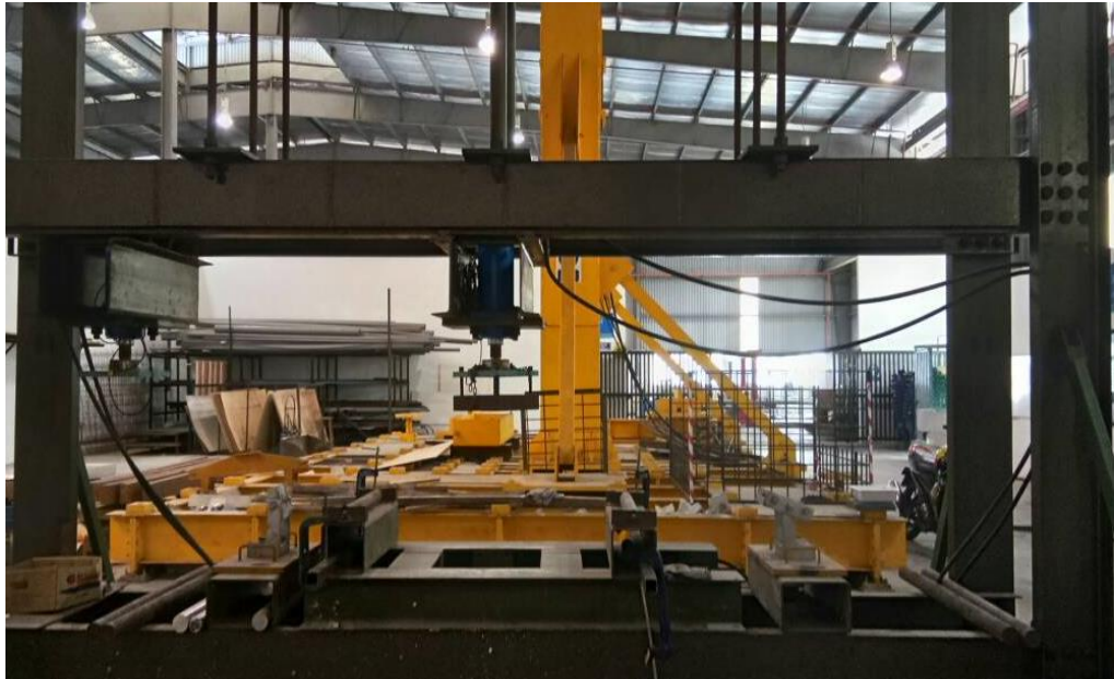
Figure 3.6 Magnus frame that used for beam testing
