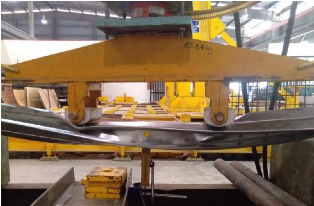
Figure 4.7 Local buckling at the middle of the beam at peak of the experiment
