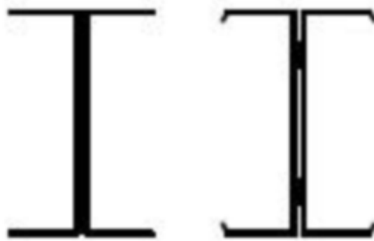
Figure 2.1 Shapes of built-up open C-section
