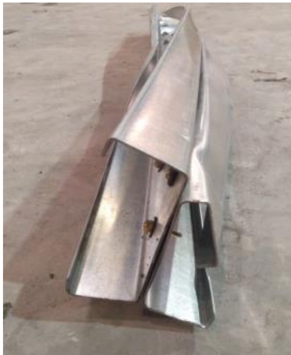
Figure 4.12 Distortional buckling occur after experiment (post – peak)
