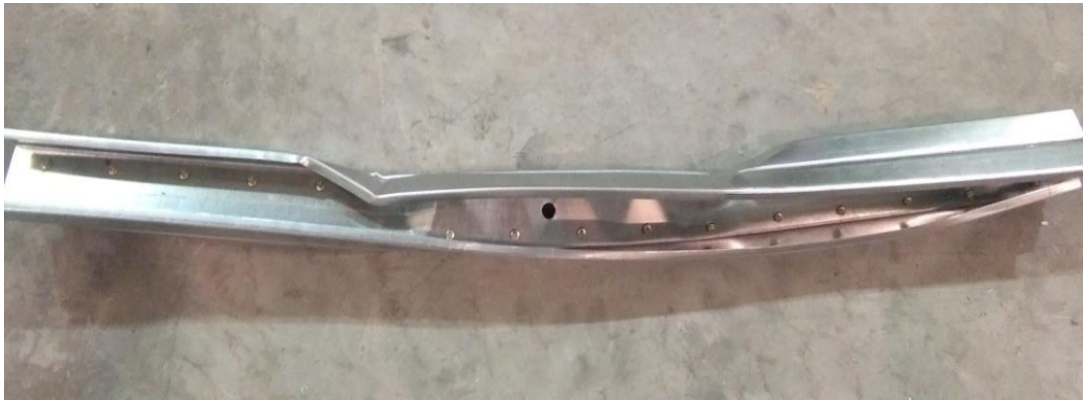
Figure 3.12 Type of buckling behavior
