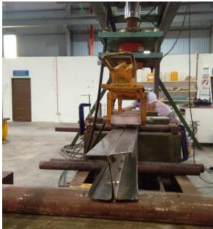
Figure 4.6 Initial local buckling during experiment (side view)
