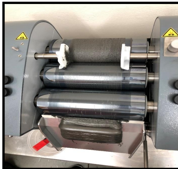
Figure 4.7: Phase separation of the existing reinforcement on the three-roll mill
