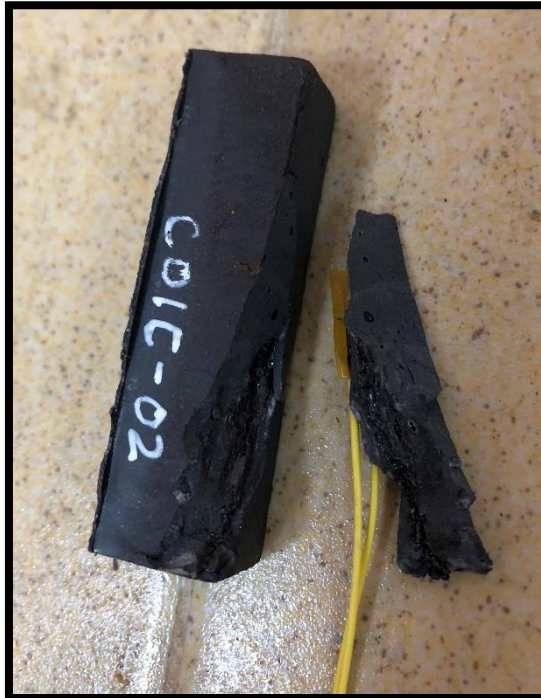
Figure 4.6: Failure pattern of compression specimen
