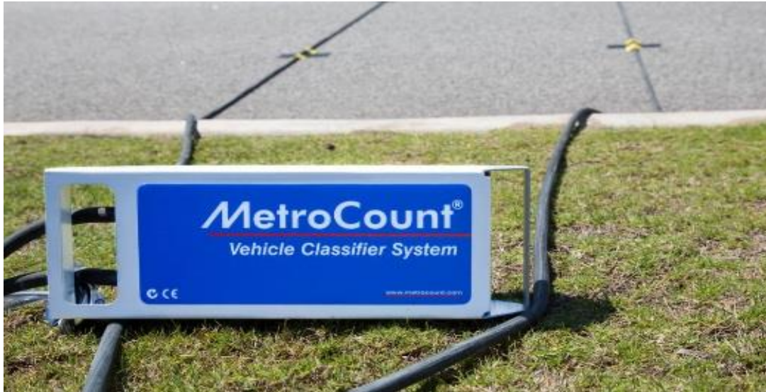
Figure 3.6 MetroCount installed on the road
