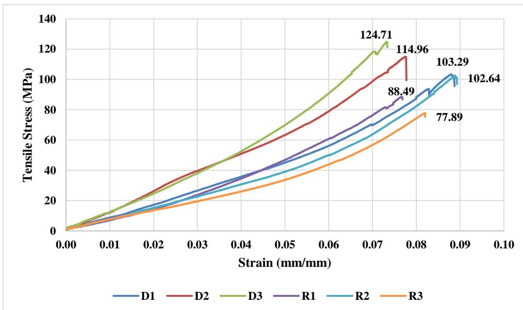
Figure 4.5 Stress vs Strain graph of Tensile Test.
