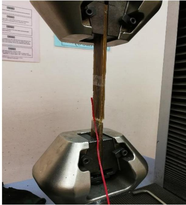
Figure 3.21 Tensile test for BFRCP.
