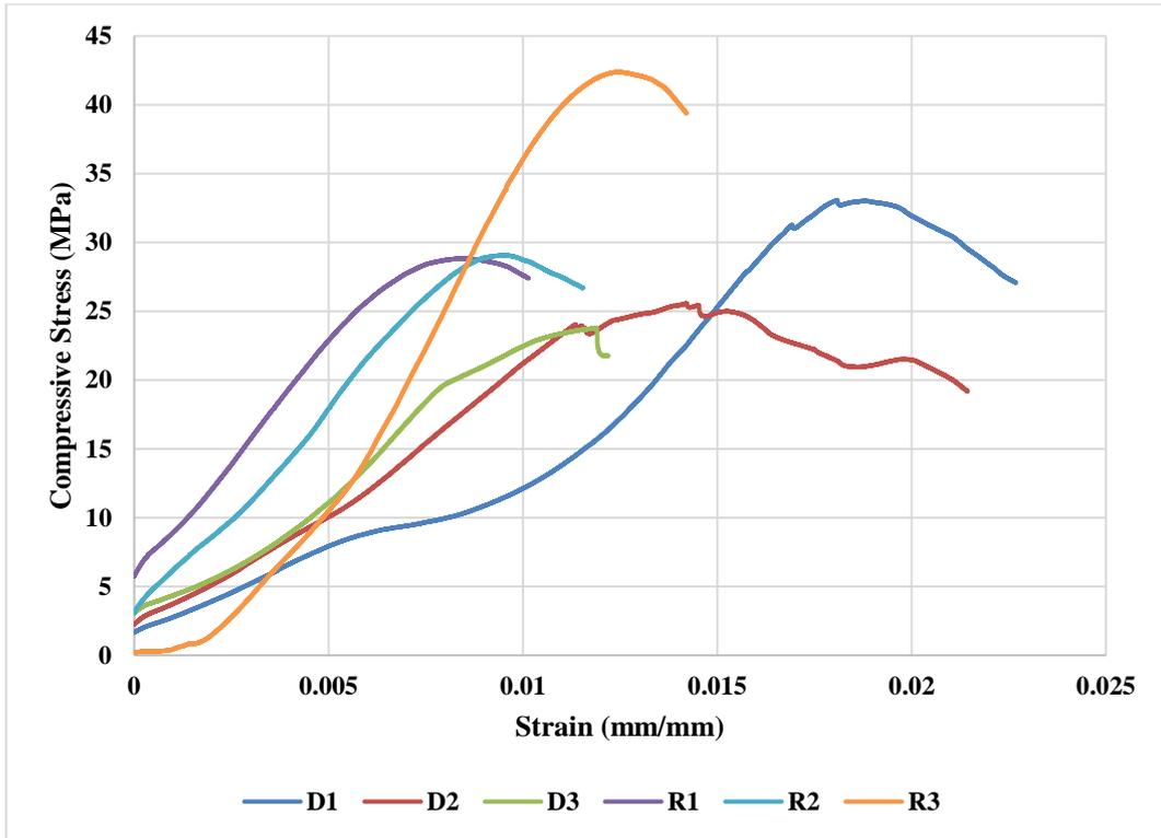
Figure 4.3 Stress vs Strain graph of Compression Test for Raw and Dried bamboo.
