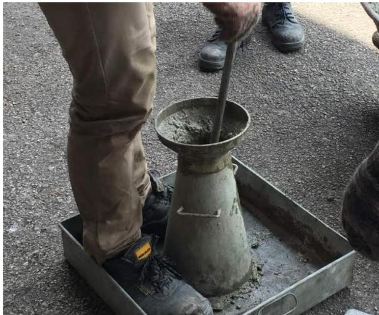
Figure 3.13 Slump test to identify the workability of fresh concrete.
