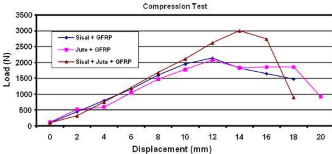
Figure 2.7 Comparison of load vs. displacement of sisal-glass fiber, jute-glass fiber, and sisal-jute-glass fiber reinforced composites.
