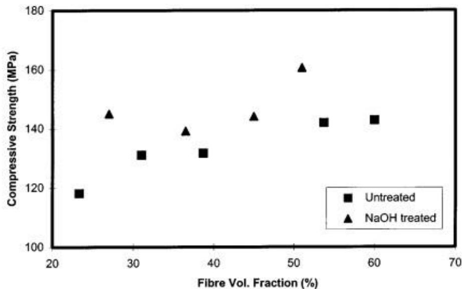
Figure 2.4 Compressive strength of sisal-epoxy composites.
