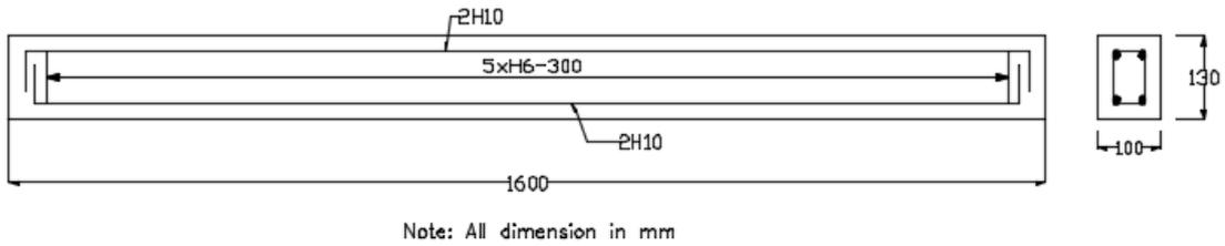
Figure 3.9 Schematic diagram for RC control beam.
