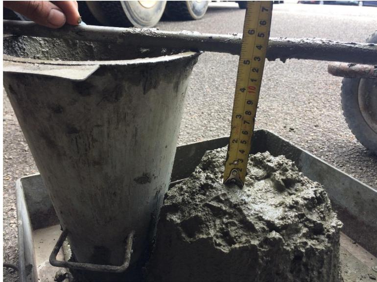
Figure 4.1 Slump test.
