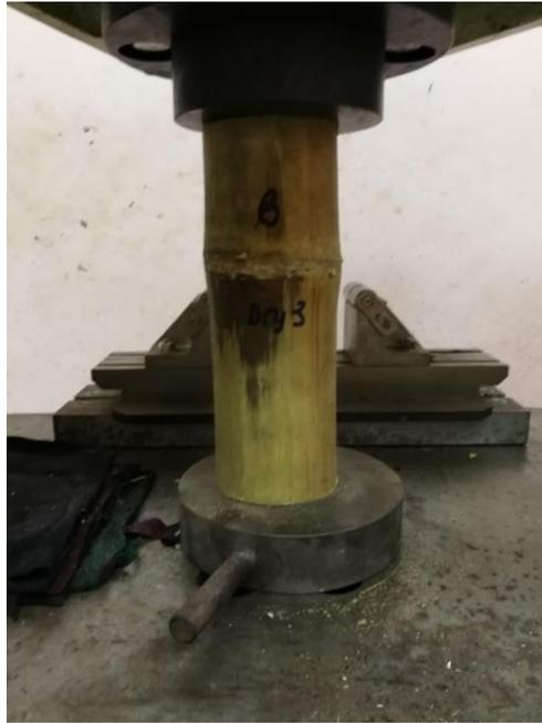
Figure 3.19 Compressive strength test of bamboo using UTM.
