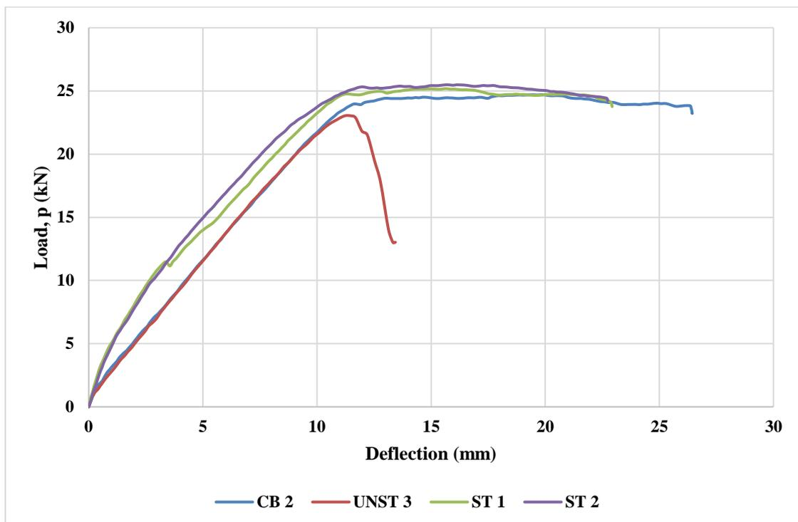
Figure 4.12 Load deflection curve of different beam specimens.
