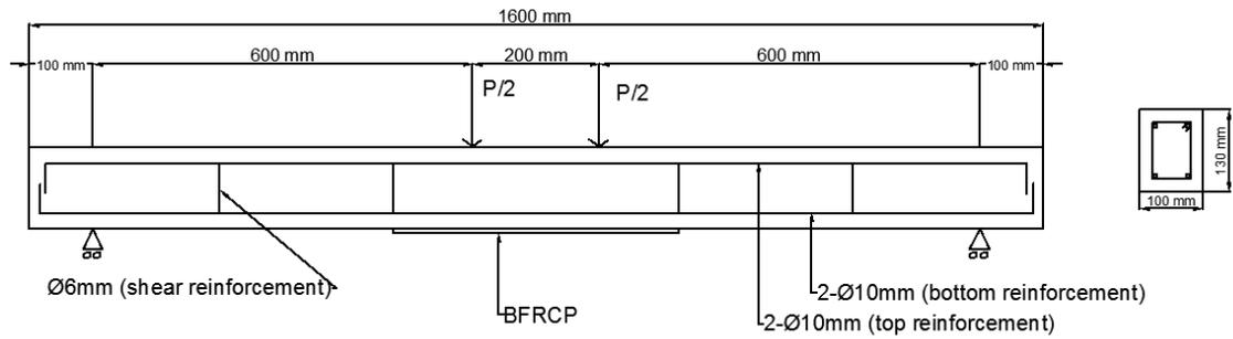
Figure 3.23 Schematic diagram of four-point loading.
