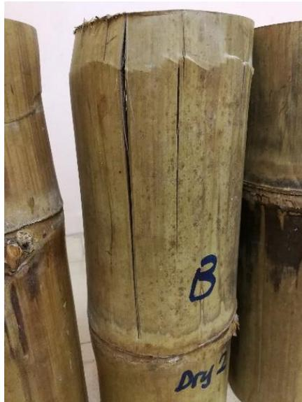
Figure 4.4 Cracking and crushing of bamboo.
