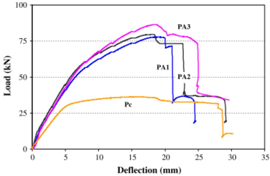
Figure 2.10 Midspan deflection of A serial beams.
