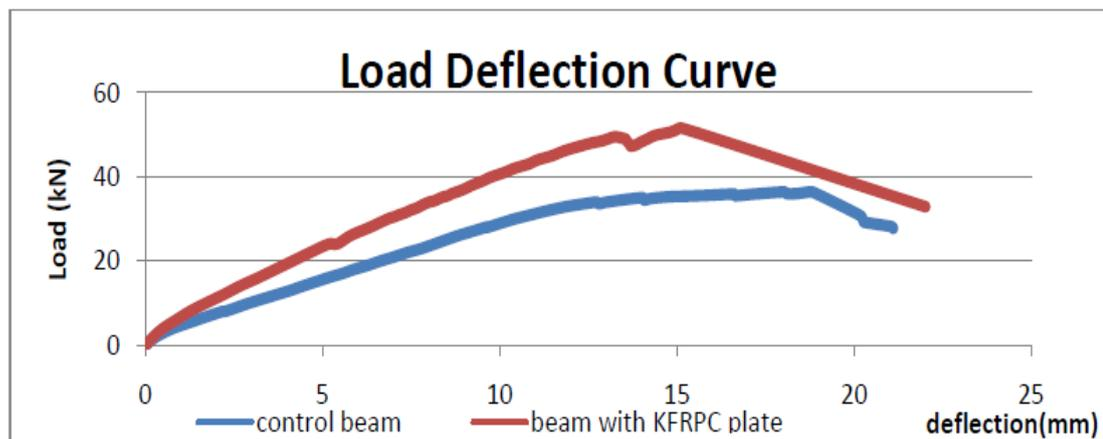
Figure 2.14 Load Deflection Curve of the different beam specimens.
