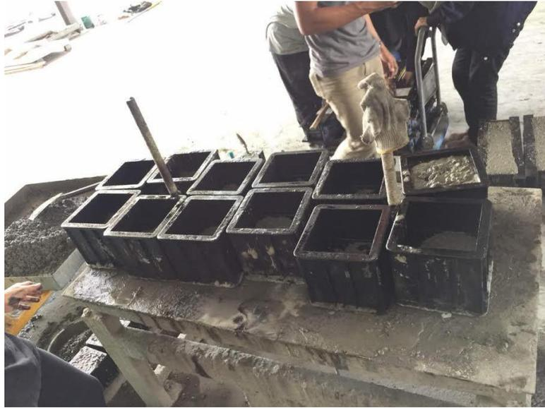
Figure 3.12 Concrete cubes sample for compressive strength tests.
