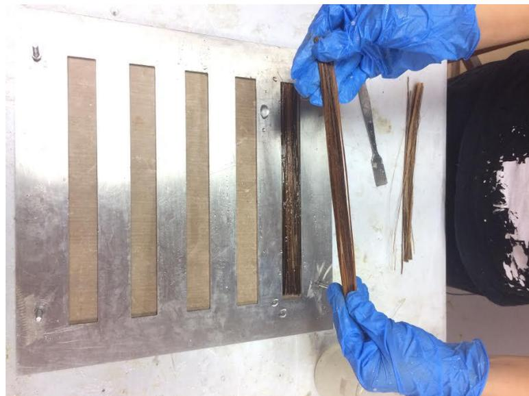
Figure 3.7 Fabricating composite plate with hand lay-up method.
