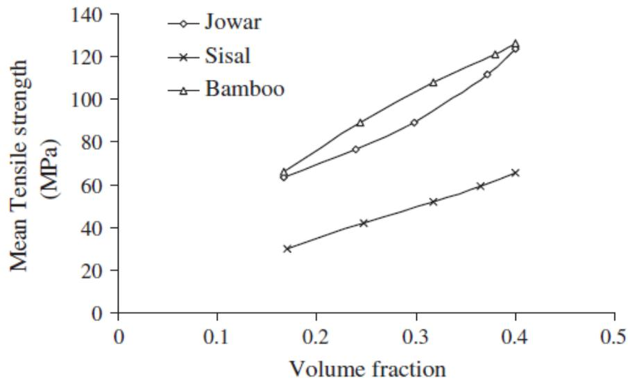
Figure 2.8 Effect of volume fraction of fiber on mean tensile strength of various natural fiber composites.
