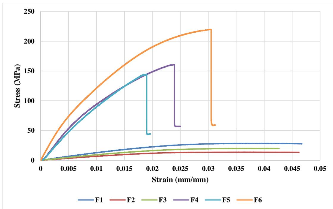
Figure 4.8 Stress-strain graph of flexural test.
