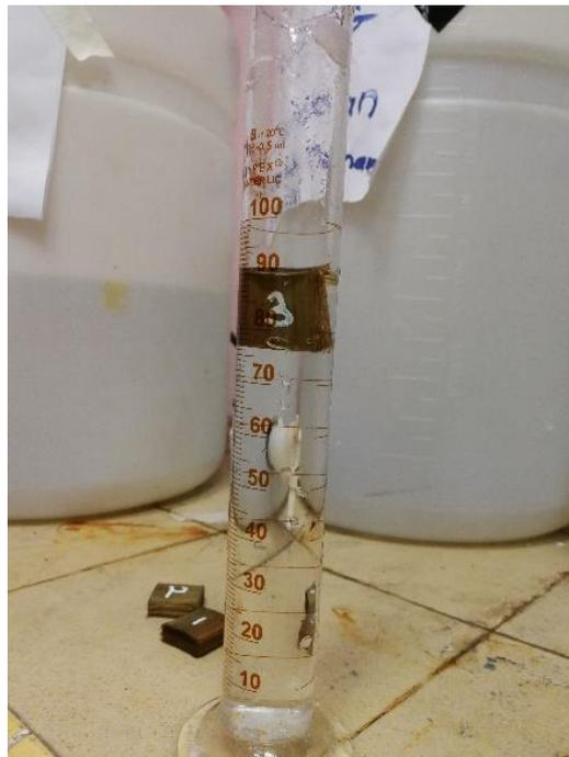
Figure 3.18 Water displacement method for determining the green volume.
