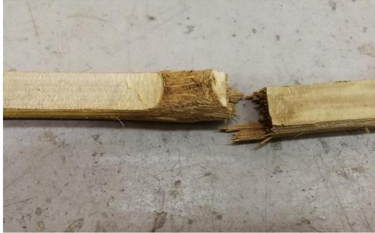
Figure 4.6 Failure of bamboo splint at node under tensile load.
