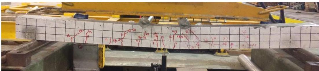
Figure 4.14 Crack patterns for CB 2.
