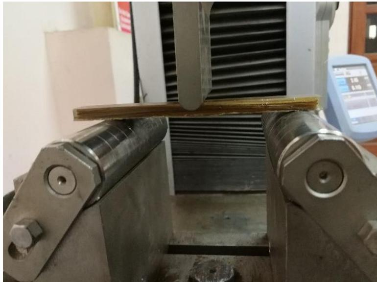
Figure 3.22 Flexural test for BFRCP.
