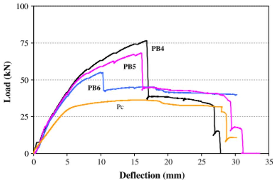
Figure 2.11 Midspan deflection of B serial beams.
