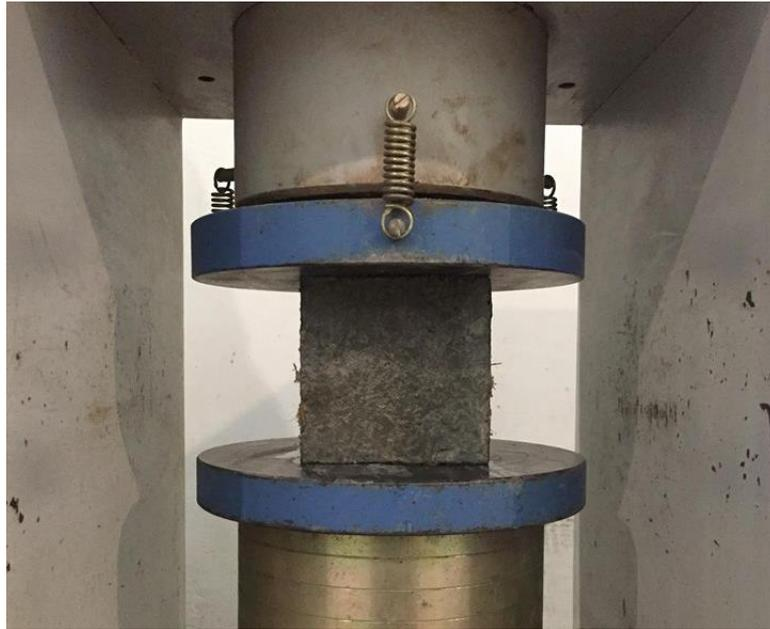
Figure 4.2 Compression test.
