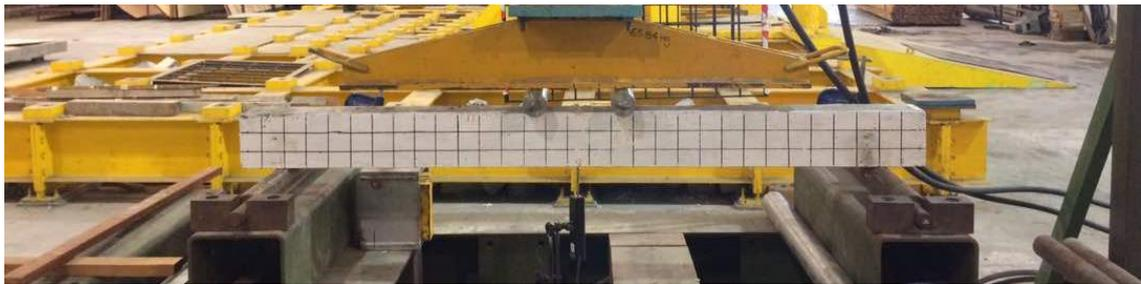
Figure 3.24 Four-point loading test setup.
