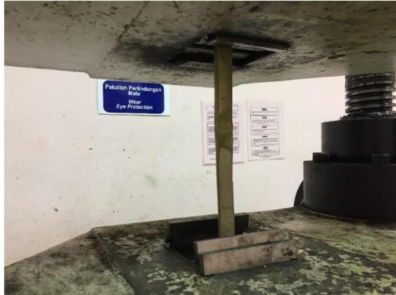
Figure 3.20 Tensile strength test of bamboo using UTM.
