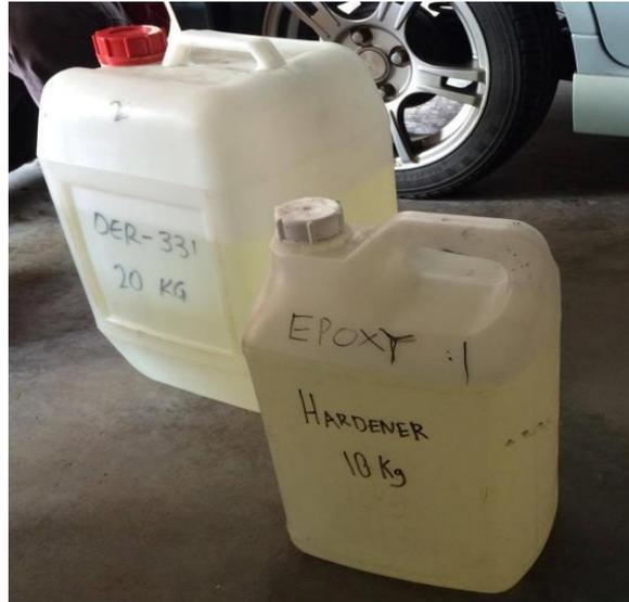
Figure 3.4 D.E.R. 331 epoxy resin and JOINTMINE 905-3S hardener.
