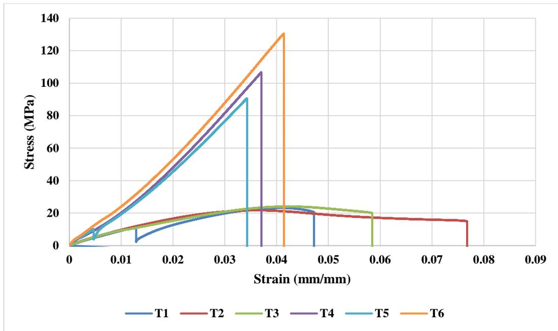
Figure 4.7 Stress-strain graph of tensile test.
