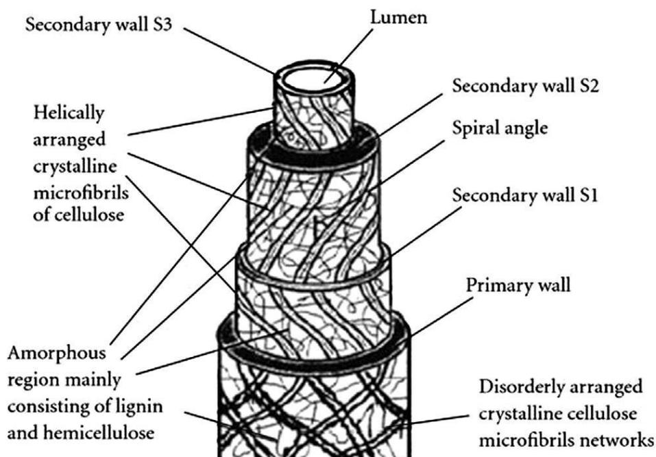
Figure 2.2 Structural constitution and arrangement of a natural vegetable fiber cell.
