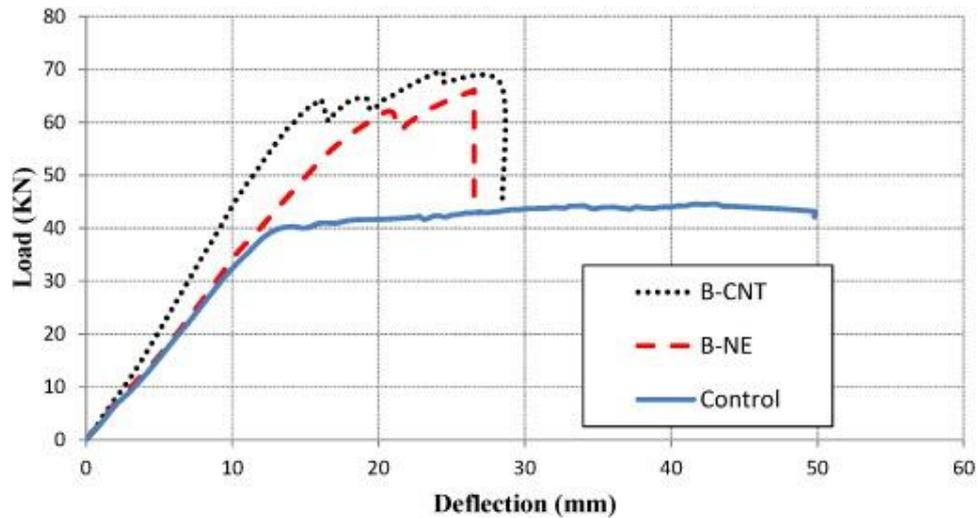
Figure 2.13 Load-deflection response of control, B-NE, and B-CNT specimens.
