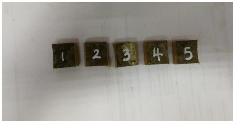
Figure 3.17 Samples for density test.
