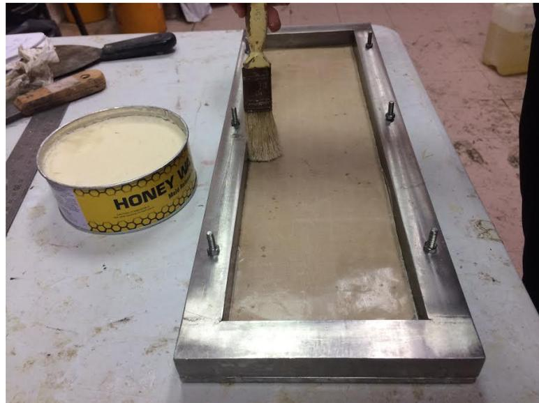
Figure 3.6 Application of mould releasing agent (honey wax).
