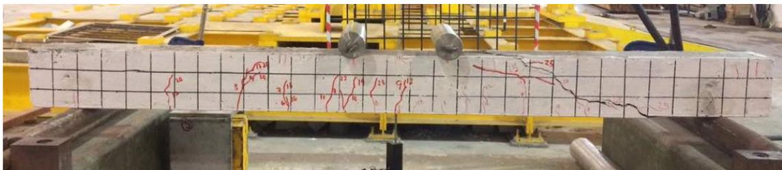
Figure 4.13 Crack patterns for CB 1.
