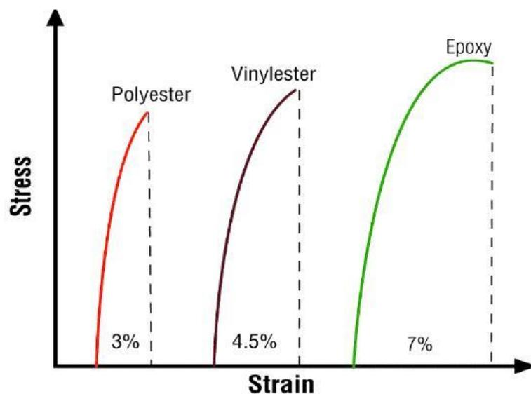
Figure 2.5 Comparison of stress-strain curve of polyester, vinylester and epoxy.
