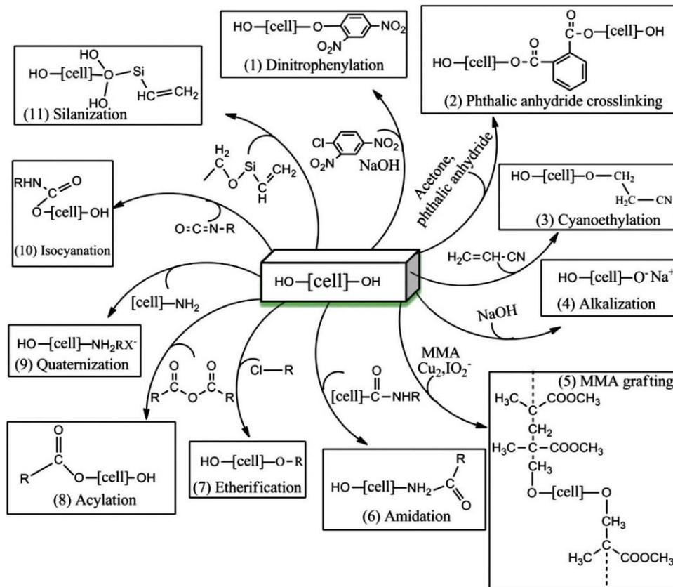
Figure 2.3 Schematic presentations of surface modifications of natural fiber.
