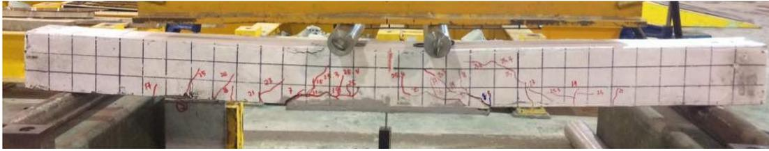
Figure 4.20 Crack patterns for ST 2.
