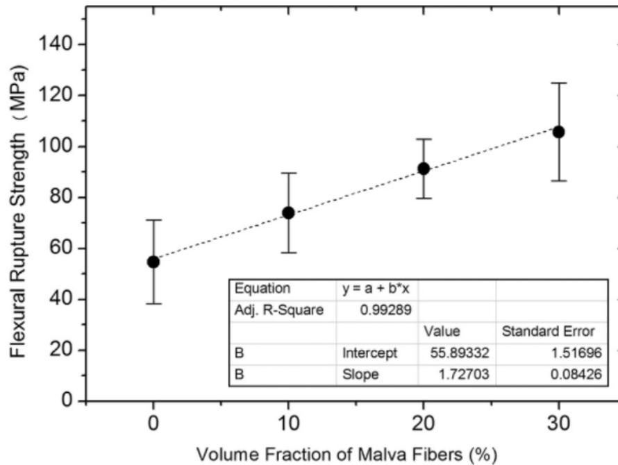
Figure 2.9 Variation of the flexural rupture strength with the volume fraction of malva fibers in epoxy composites.
