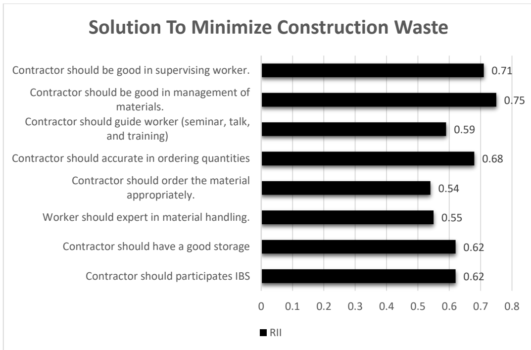
Figure 4-14: RII Values of Solution to Minimize Construction Waste
