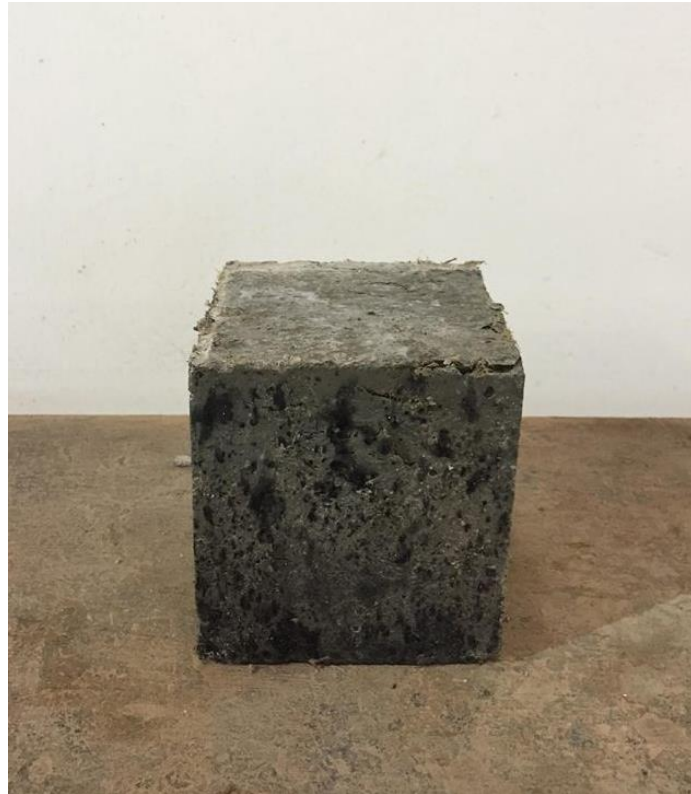
Figure 4.10: Failure pattern of bamboo fibre reinforced concrete cube
