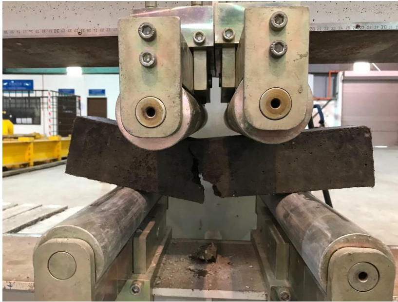
Figure 4.12: Failure pattern of normal structural beam
