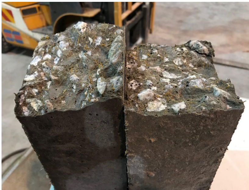
Figure 4.13: Fibre bridging inside the concrete
