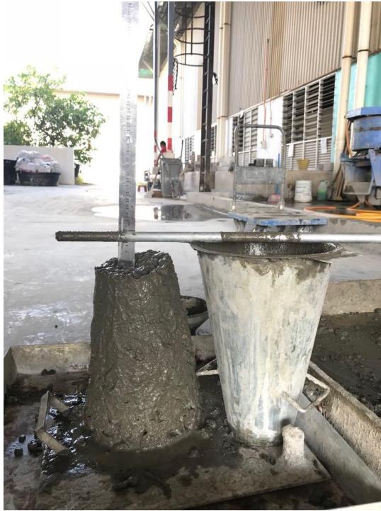
Figure 4.5: Slump Test for Control Mix
