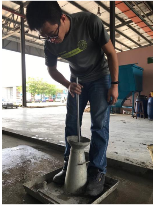
Figure 3.17: Blowing tamping rod for compaction
