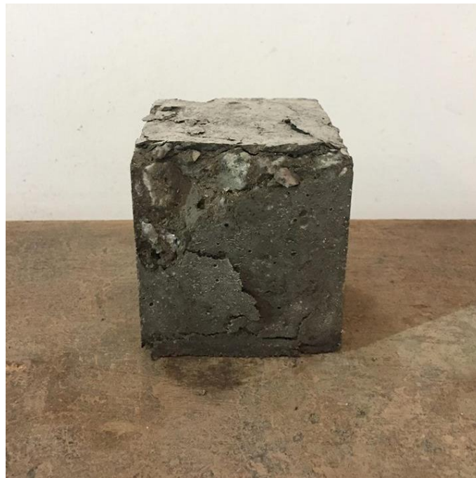
Figure 4.9: Failure pattern of normal concrete cube
