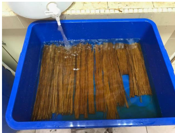
Figure 3.9: Neutralization of bamboo fibers
