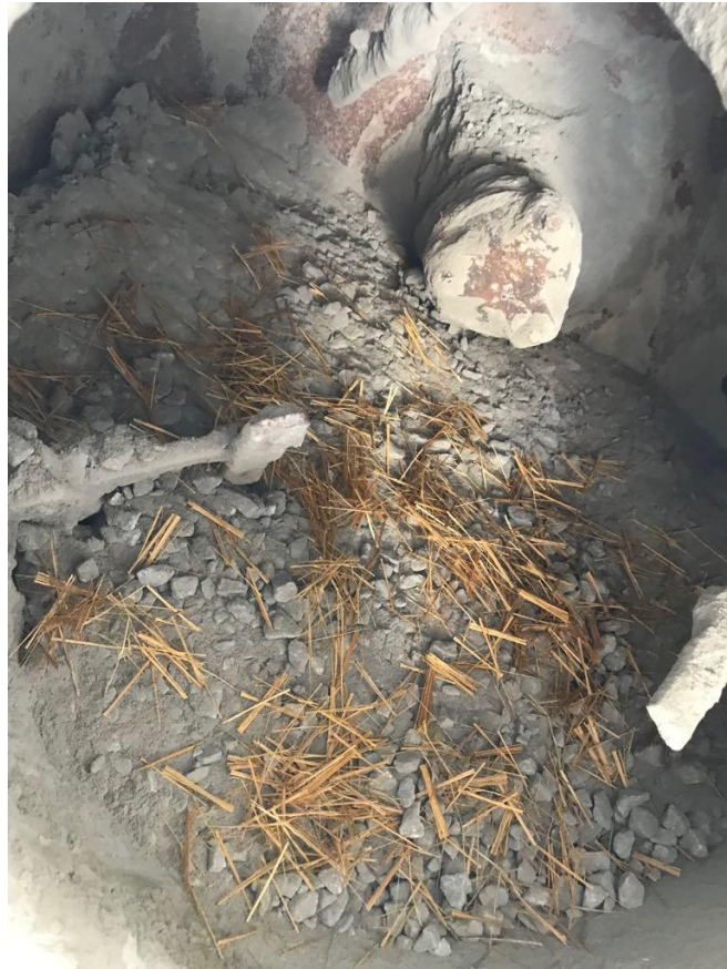
Figure 3.15: Fibre disperse in concrete mixer
