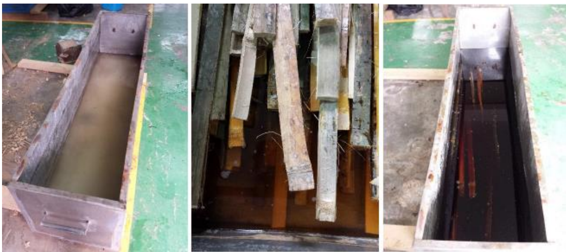
Figure 3.7: Alkaline retting process
