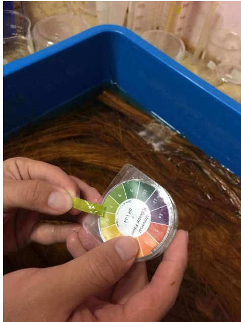
Figure 3.10: Measuring the PH value of bamboo fibre
