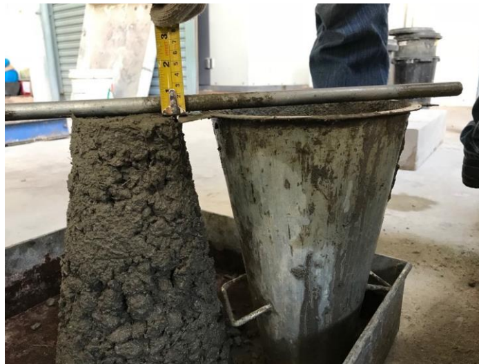
Figure 4.6: Slump Test for Fibre Concrete Mix
