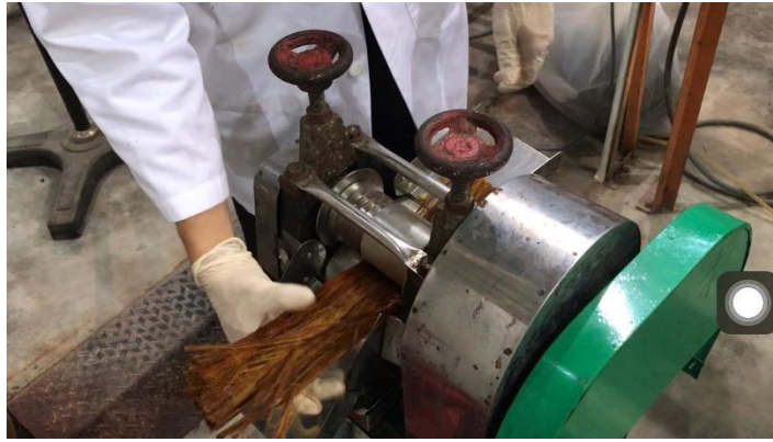
Figure 3.8: Roll milling process
