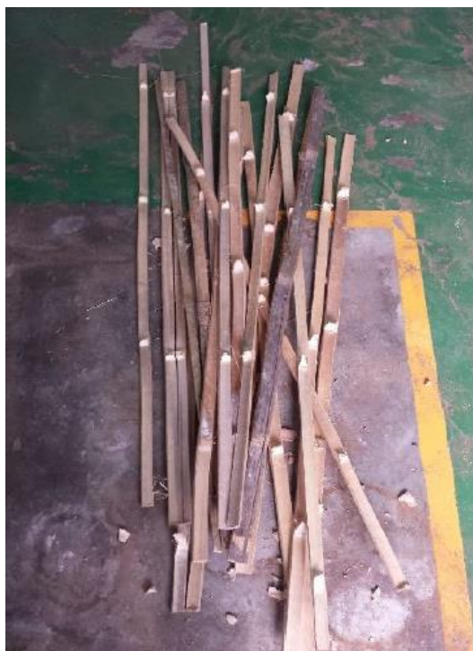
Figure 3.6: Bamboo culm cleaved into splits
