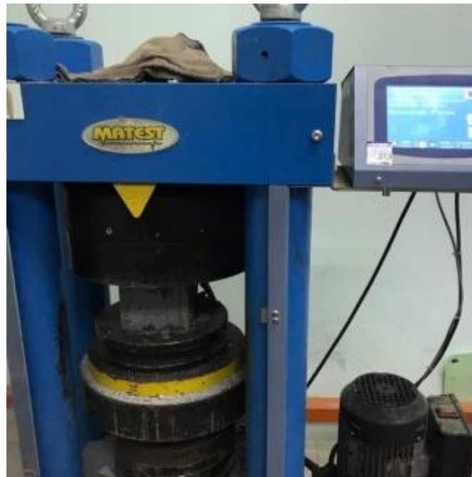
Figure 3.4 Compressive test in progress.
