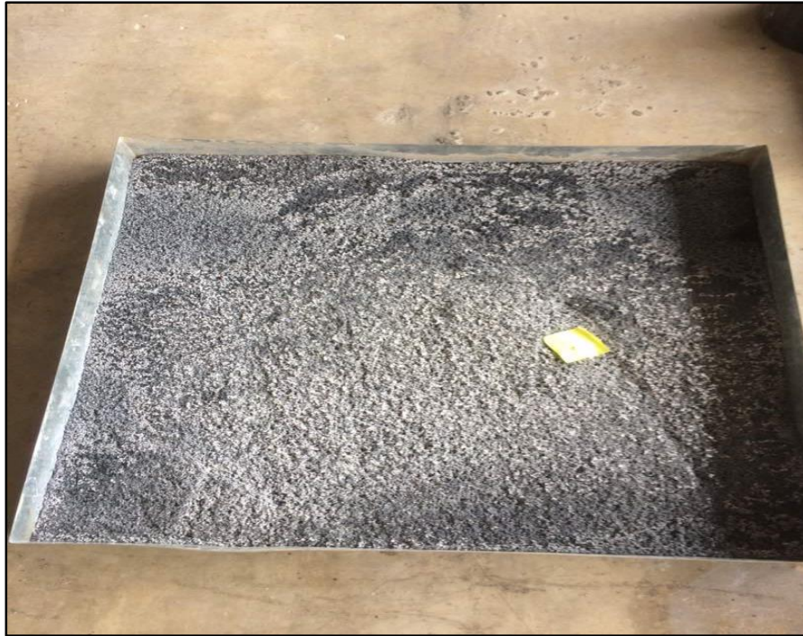
Figure 4.2 Appearance of Waste Crumb Tyre Particles After subjected to Pre-Treatment Process
