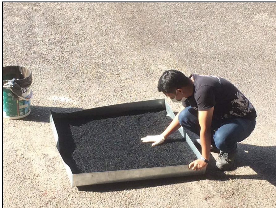
Figure 4.1 Appearance of Waste Crumb Tyre Particles before Treatment Subjected to Pre-Treatment Process.
