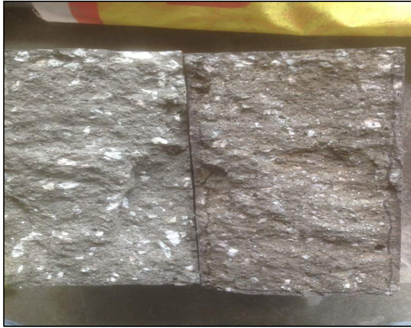
Figure 4.31 Visual Appearance of the Splitting Surface Cylinder after \text{AgNO}_3 Spray Method for UHPC-40 at 28 days
