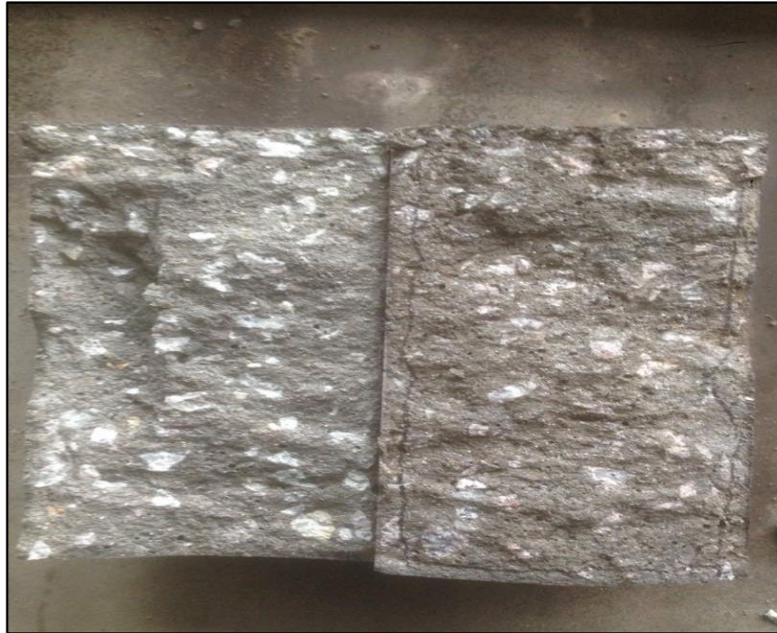
Figure 4.30 Visual Appearance of the Splitting Surface Cylinder after \text{AgNO}_3 Spray Method for UHPC-20 at 28 days
