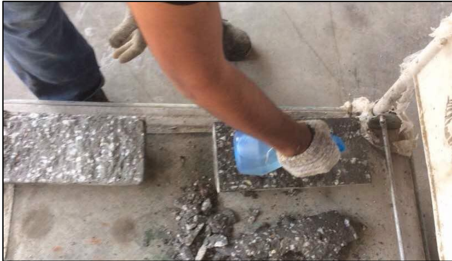
Figure 3.14 Spray Silver Nitrate ( \text{AgNO}_3 )
