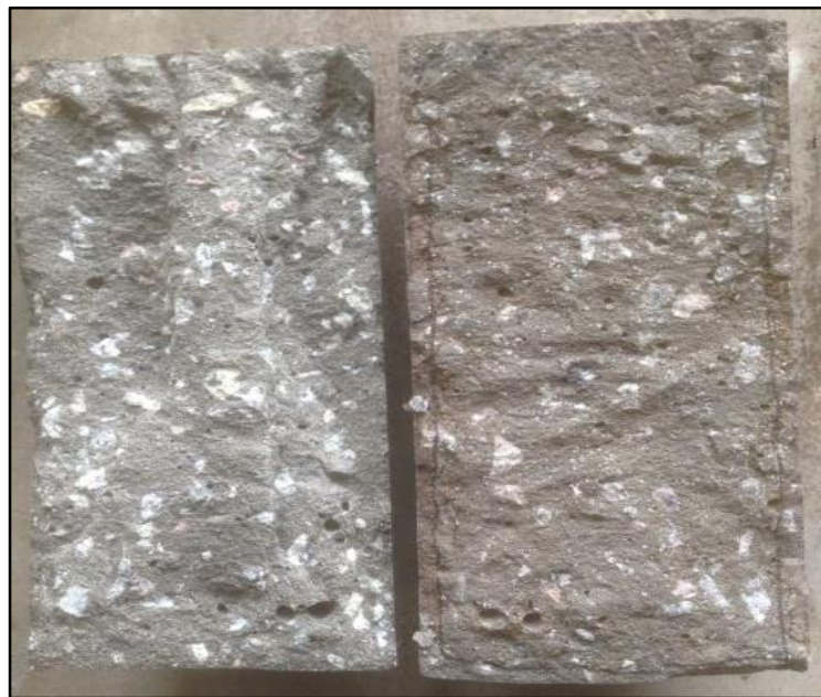
Figure 4.29 Visual Appearance of the Splitting Surface Cylinder after \text{AgNO}_3 Spray Method for Plain UHPC at 28 days
