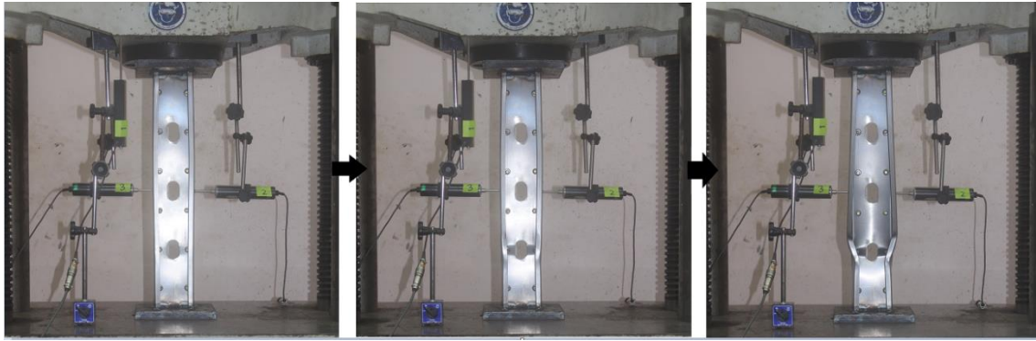
Figure 4.17 Buckling behaviour of specimen BC103-1.2-A5 (Initial, peak, post)
