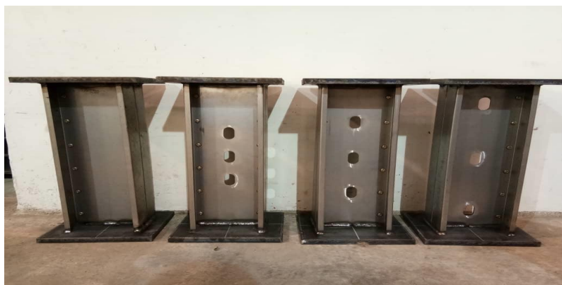
Figure 2.2 Show the built-up c-sections specimen
