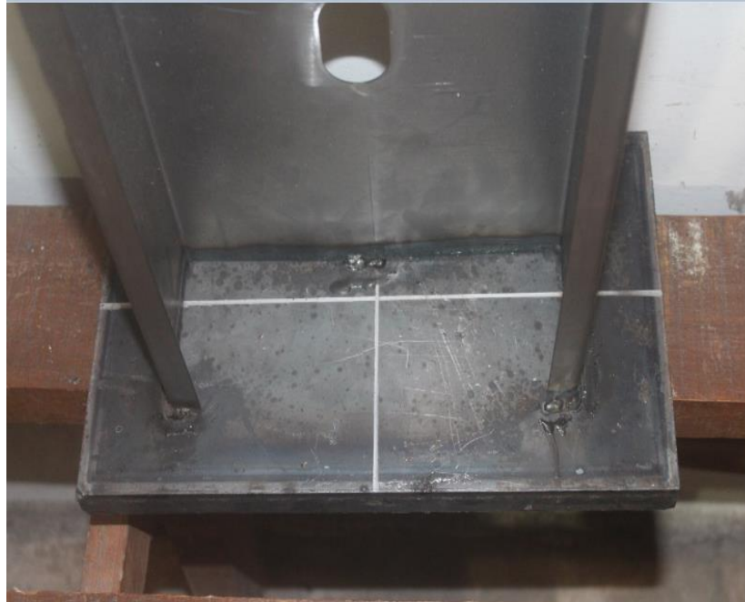
Figure 3.11 Specimen welded at bottom support
