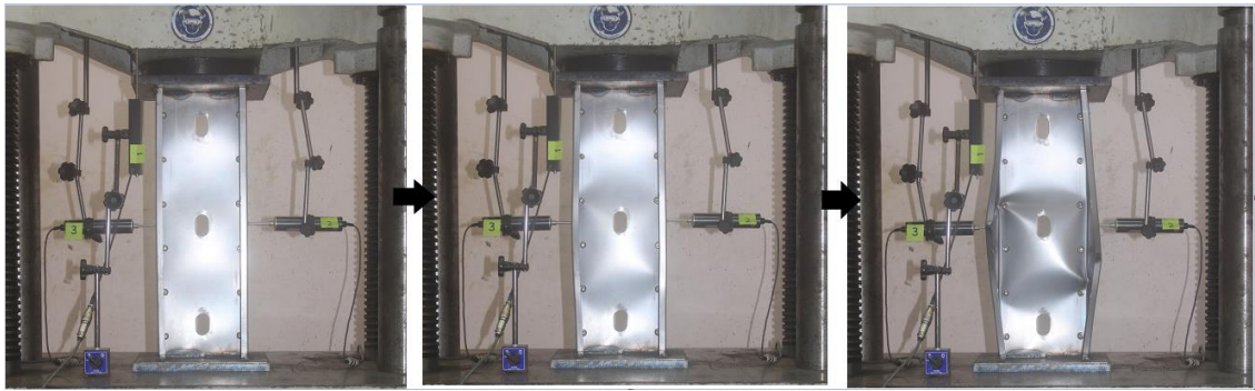
Figure 4.14 Buckling behaviour of specimen BC203-1.2-A8 ( Initial, peak, post)
