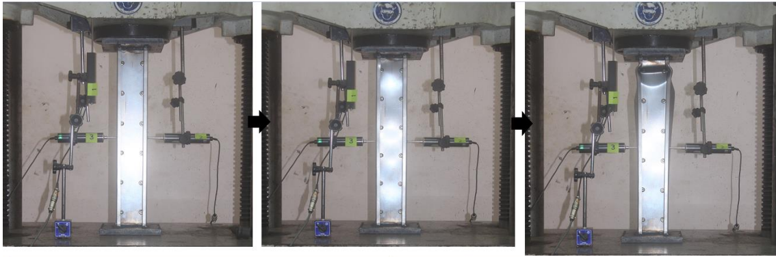
Figure 4.15 Buckling behaviour of specimen BC103-1.2-A1 (Initial, peak, post)
