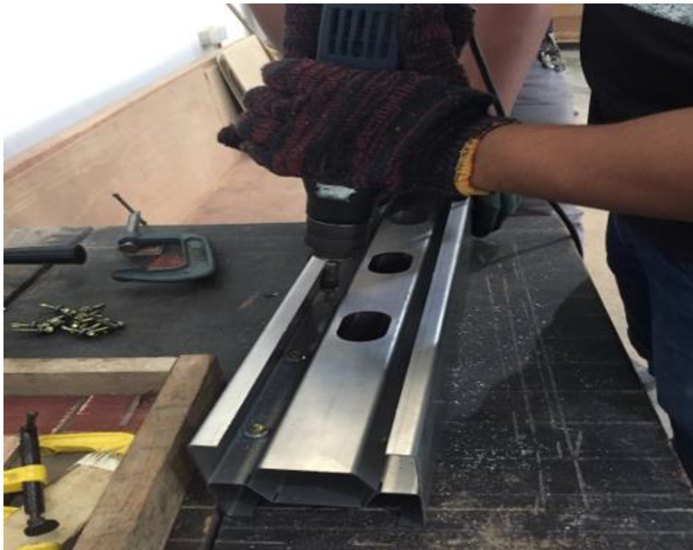
Figure 3.9 Forming the built-up specimen with self-drilling screw
