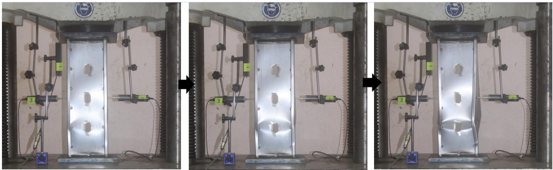
Figure 4.13 Buckling behaviour of specimen BC203-1.2-A5 ( Initial, peak, post)
