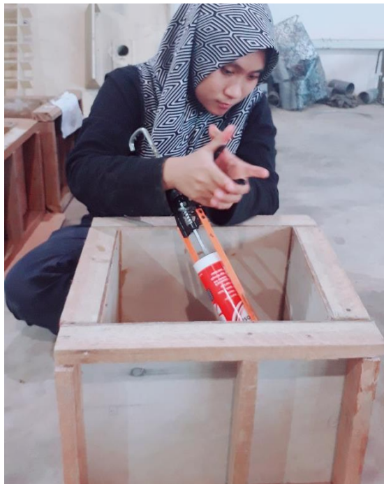
Figure 3.7 Work to Cover the Wood Mould with Silicone Gel
