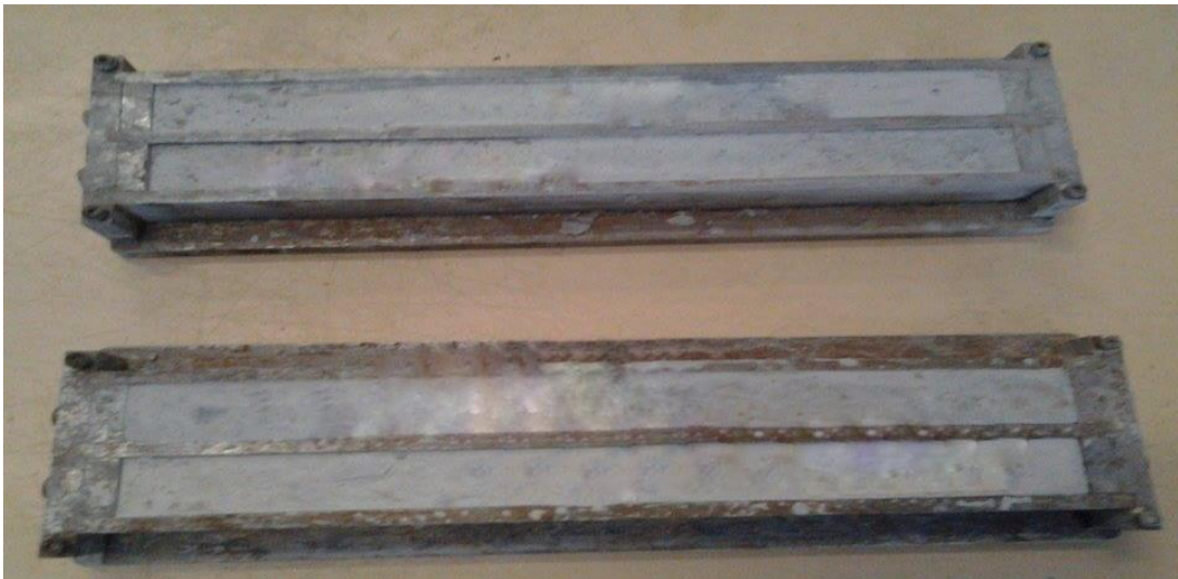
Figure 3.11 Steel Fibre Concrete in Steel Mould
