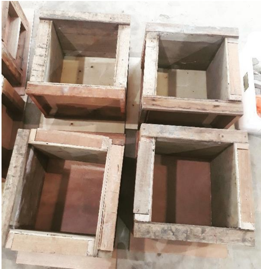
Figure 3.8 Wood Mould for Heat of Hydration Test
