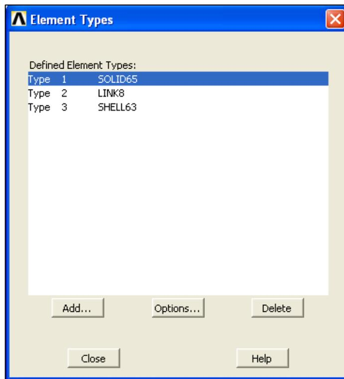
Figure 3.7: Element types chosen in analysis.
