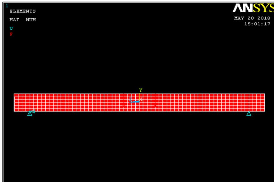
Figure 3.23: Side view of beam that had been applied with supports and loads.
