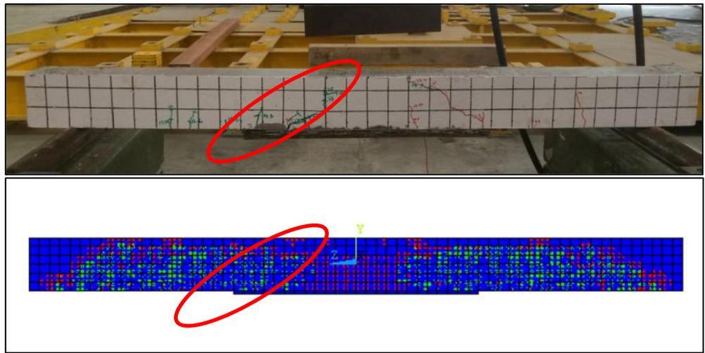
Figure 4.12: Crack pattern of RCS1 (comparison)
