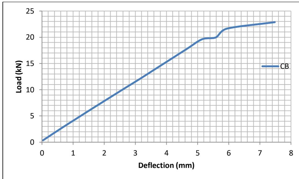
Figure 4.1: Load-deflection curve of control beam (CB)
