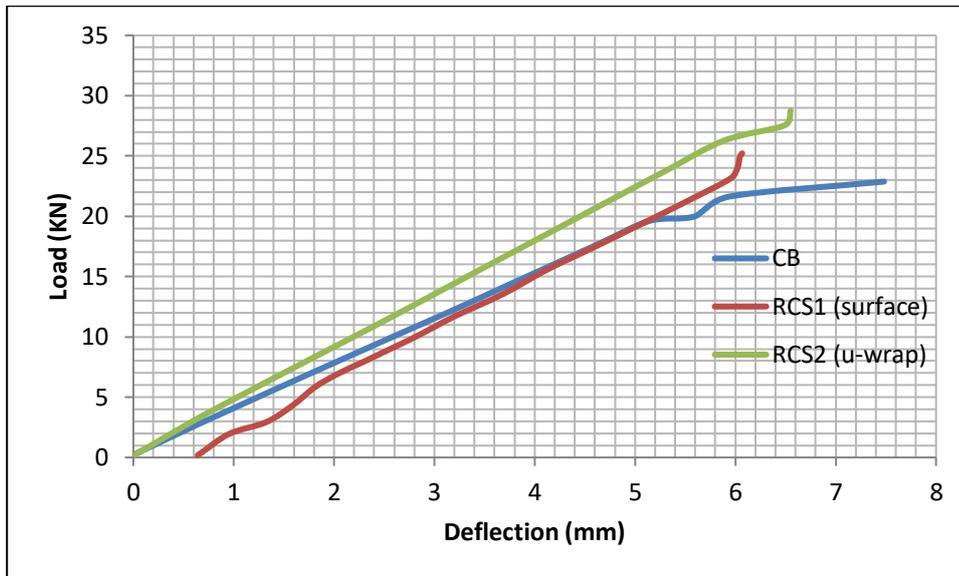
Figure 4.17: Comparison of load-deflection curve of all beam models
