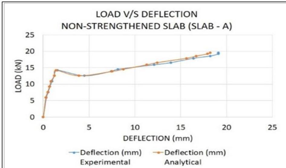
Figure 2.13: Load v/s Deflection curve for Slab – A (Non-Strengthened)
