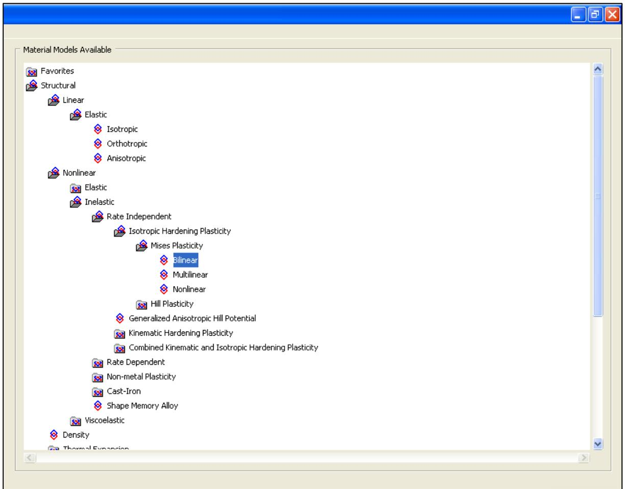
Figure 3.8: Materials properties of model analysis.
