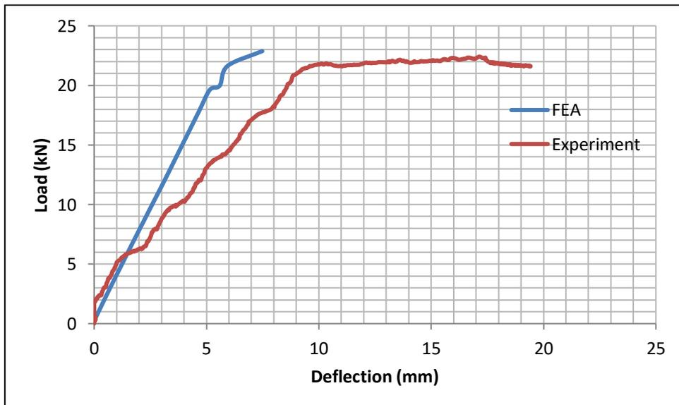
Figure 4.5: Load-deflection curve of CB (comparison)
