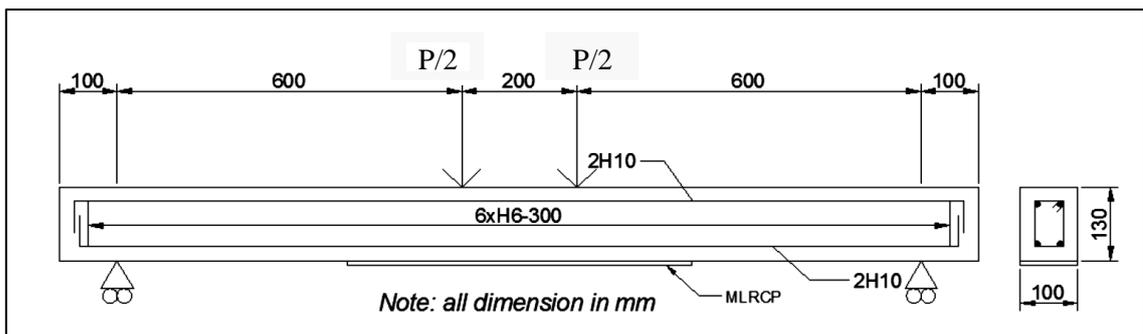
Figure 3.3: Schematic diagram of RC beam with surface strengthening.
