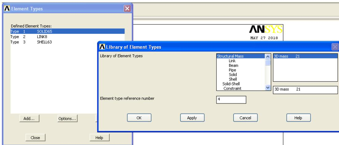
Figure 3.6: Material code for concrete strength G25, SOLID 65.
