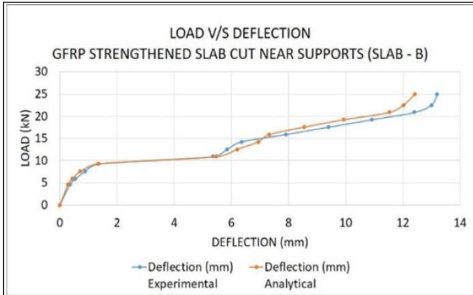
Figure 2.14: Load v/s Deflection curve for Slab – B (GFRP Strengthened – cut near supports)
