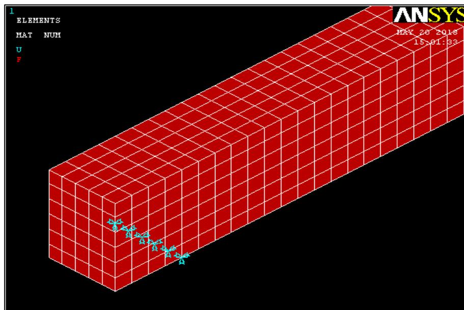
Figure 3.24: Support that had been restrained with three degree of freedom.
