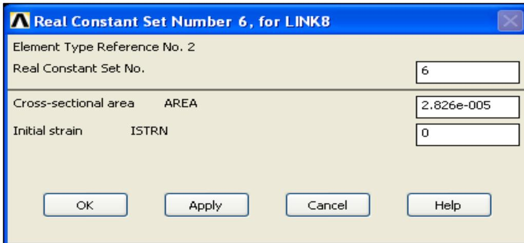
Figure 3.10: Input data of area of the steel to define the real constant.
