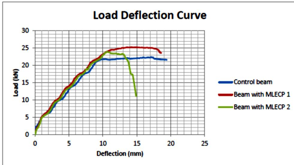
Figure 2.7: Load deflection curve of the different beam specimen.
