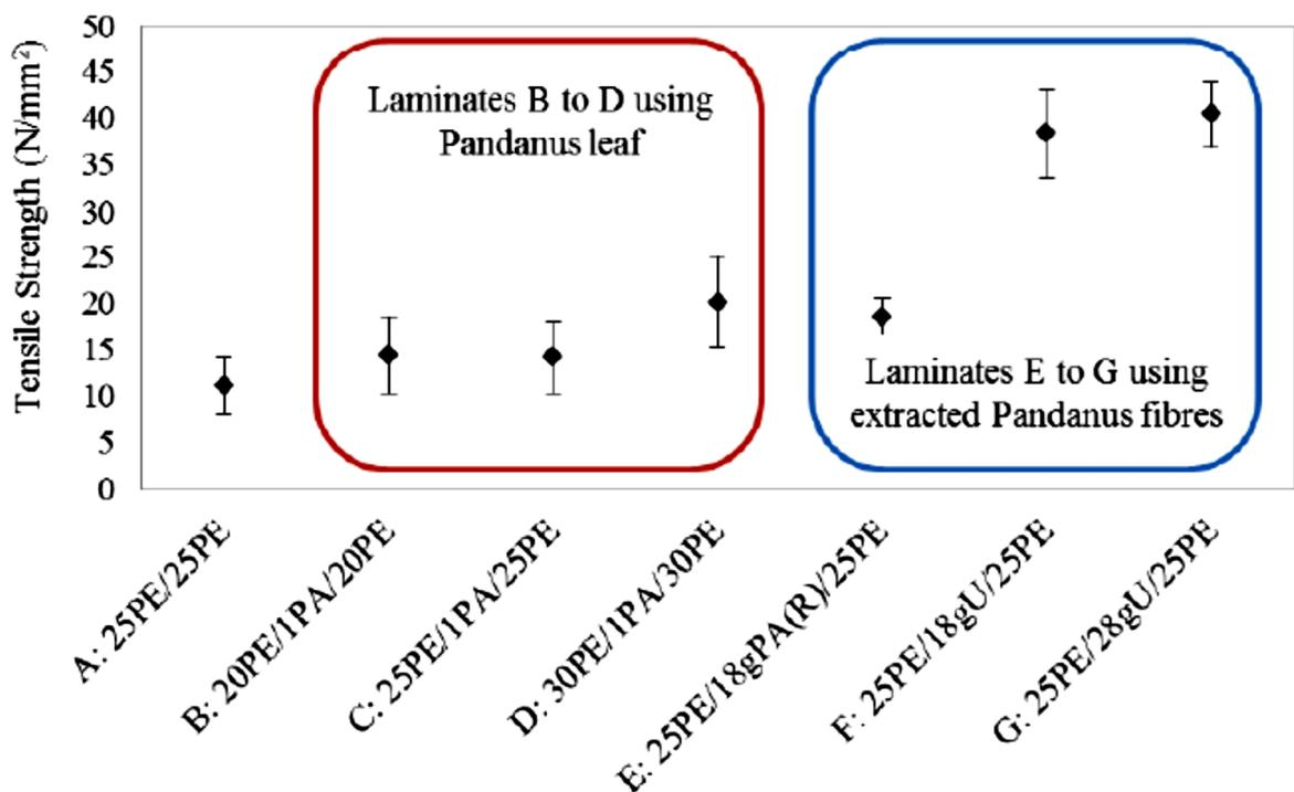
Figure 2.4: The variation of the tensile strength of the entire PA (leaf and fibres) reinforced PE. Laminate A (neat PE) is included for comparison.
