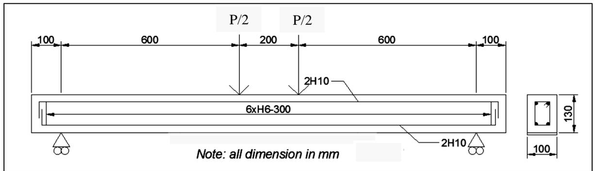
Figure 3.1: Schematic diagram of RC beam
