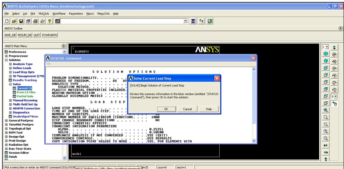
Figure 3.26: Interactive window of initializing the analysis
