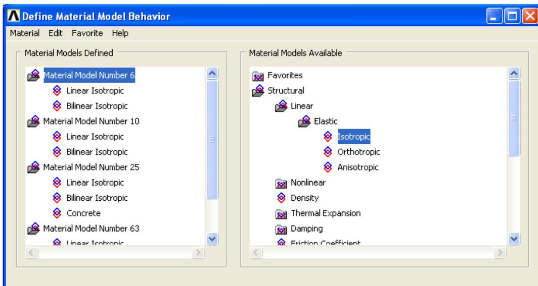
Figure 3.9: Summary of materials assigned to the element in analysis.
