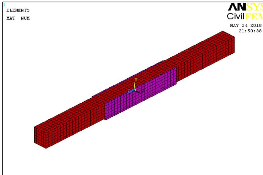
Figure 3.22: RC beam strengthened by MLECP (U-wrap)
