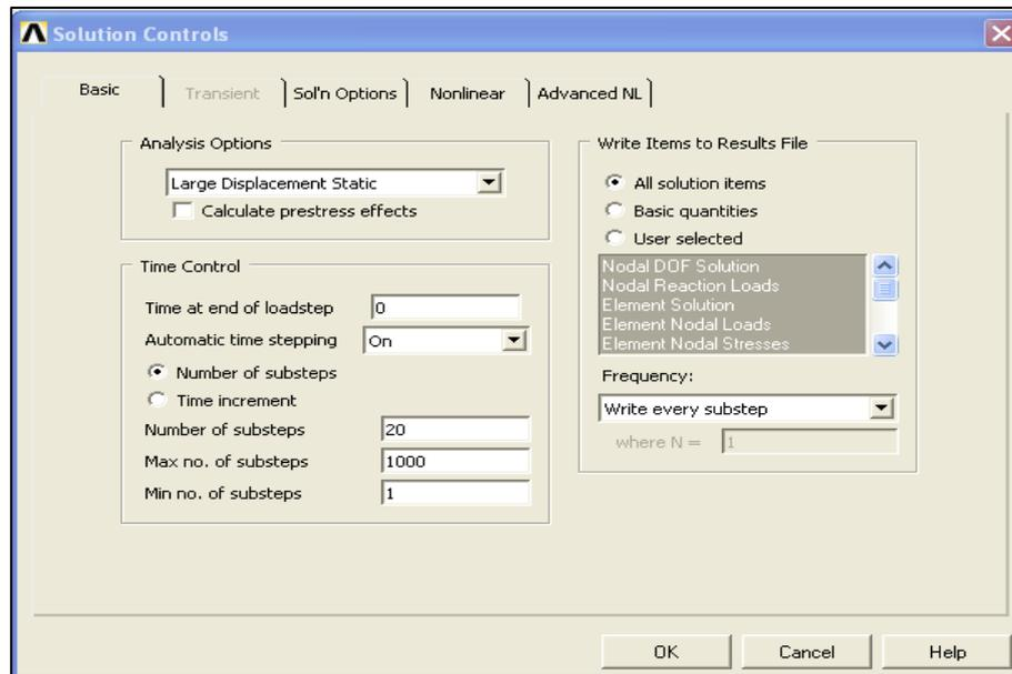
Figure 3.25: Solution controls table to set the option for load applying
