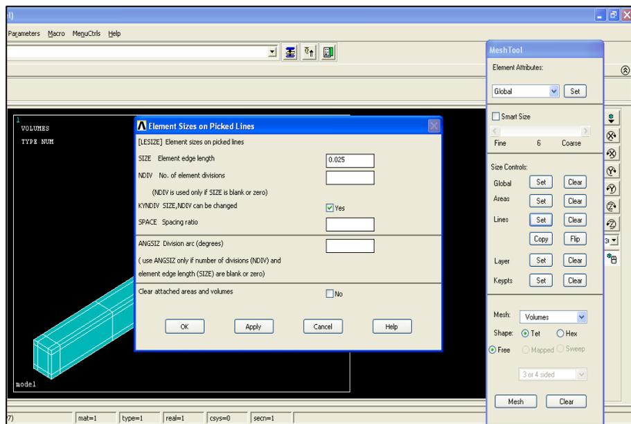
Figure 3.16: Size used for element size on picked lines.
