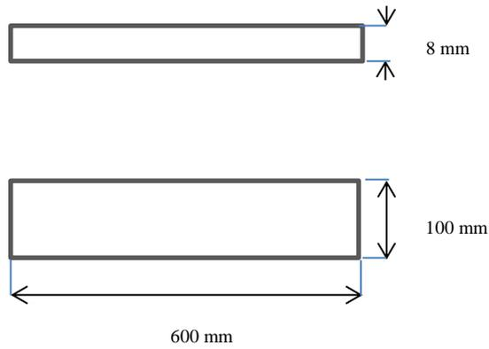
Figure 3.2: Schematic diagram of Mengkuang Leaves Epoxy-composite Plate
