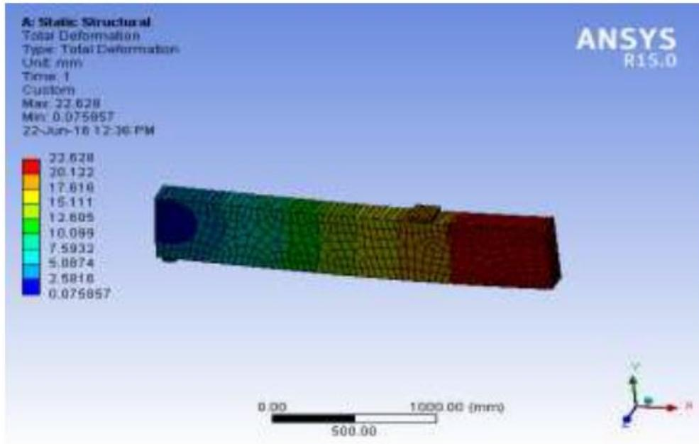
Figure 2.16: Deformation Shape of ARFP (sides+bottom)
