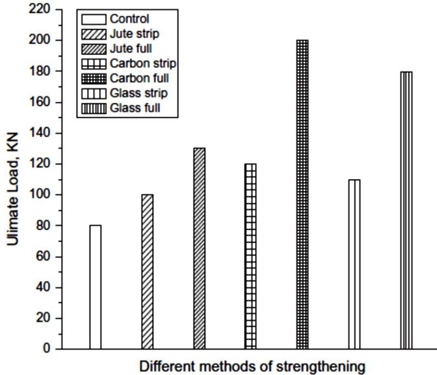
Figure 2.9: Ultimate load carrying capacity of beams
