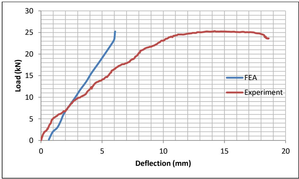
Figure 4.11: Load-deflection curve of RCS1 (comparison)
