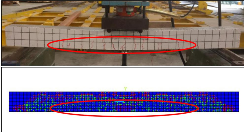
Figure 4.6: Crack Pattern of CB (comparison)
