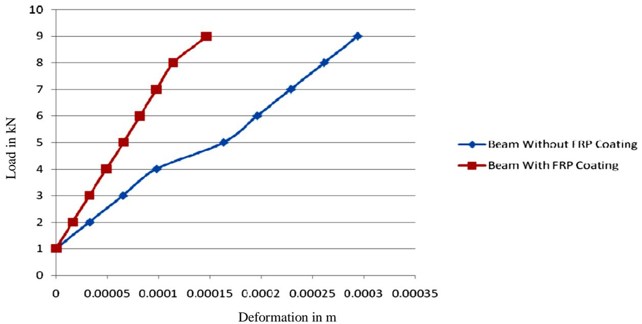
Figure 2.10: Comparison of the beams in terms of load deflection
