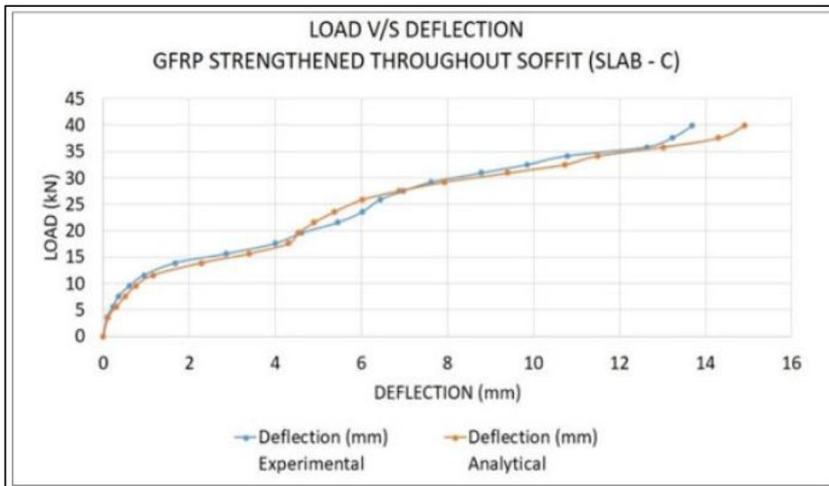
Figure 2.15: Load v/s Deflection curve for Slab – C (GFRP Strengthened – throughout the soffit)
