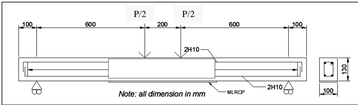
Figure 3.4: Schematic diagram of RC beam with U-wrap strengthening method.
