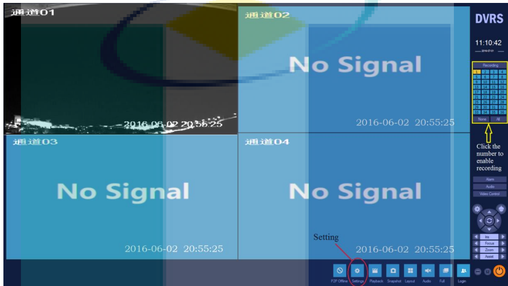
Figure 3.15 Recording control panel.
