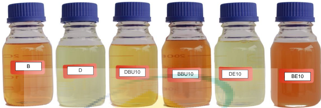
Figure 3.3 Mineral diesel (D), palm biodiesel (B), DBu10 (90 % diesel + 10% butanol), BBU10 (90 % palm biodiesel + 10% butanol), DE10 (90 % diesel + 10% ethanol), and BE10 (90 % palm biodiesel + 10% ethanol)
