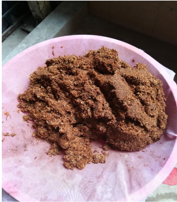
Figure 3.7 Soaked wood dust was filtered
