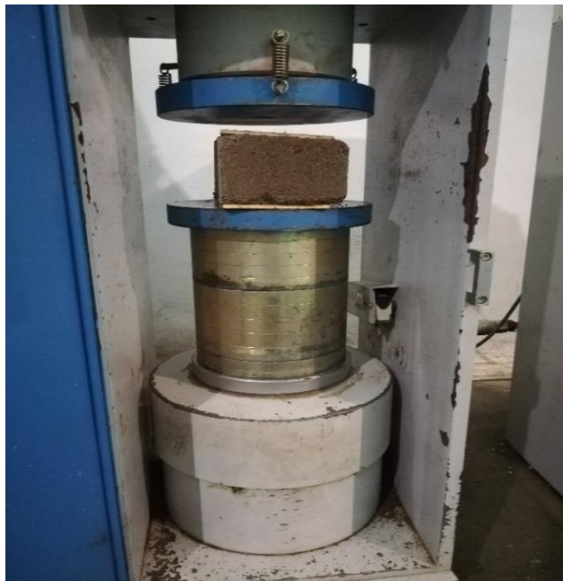
Figure 3.18 Sample placed on the testing machine
