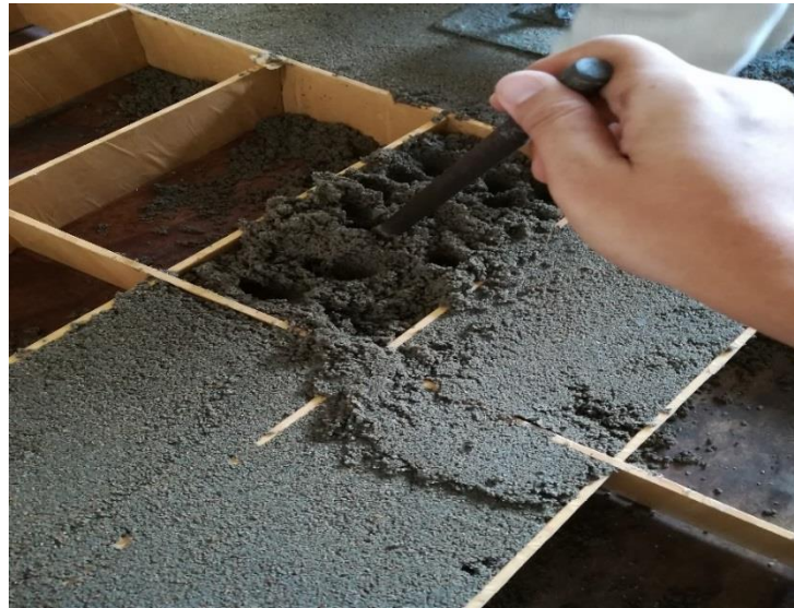
Figure 3.13 Sample was compacted using steel rod
