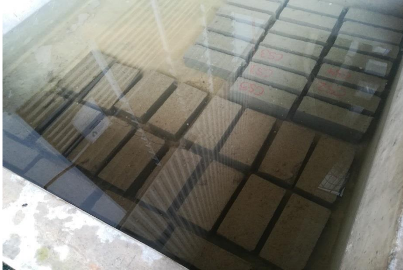
Figure 3.16 Water curing process
