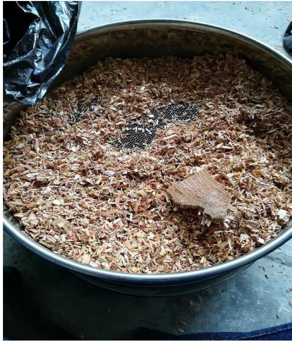
Figure 3.5 Sieve process of wood dust
