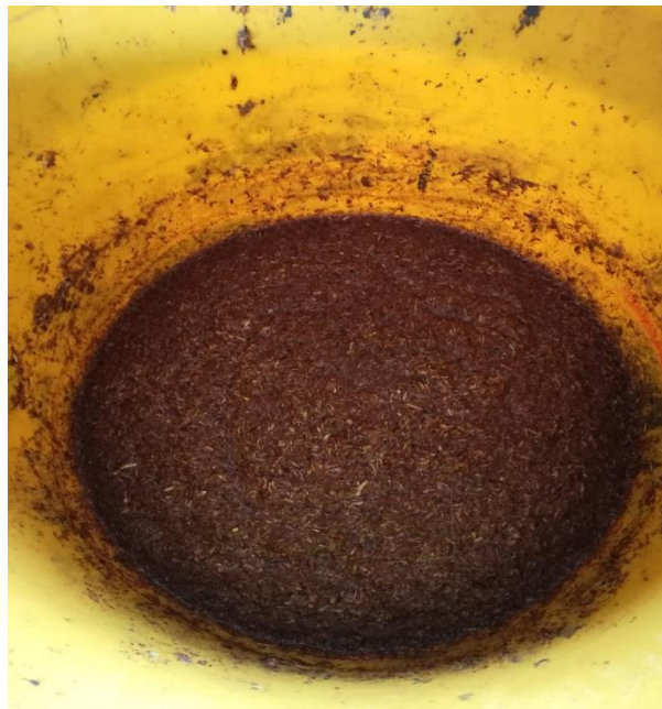
Figure 3.6 Wood dust soaked with water
