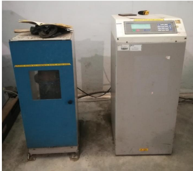
Figure 3.17 Compressive strength machine
