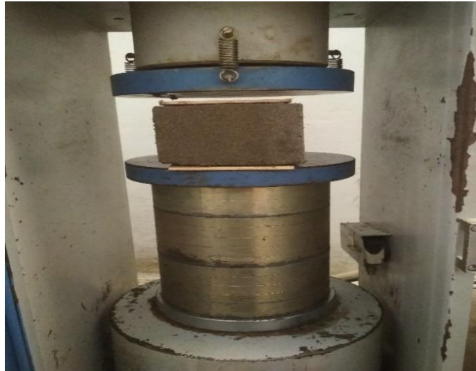
Figure 3.15 Process of compression test
