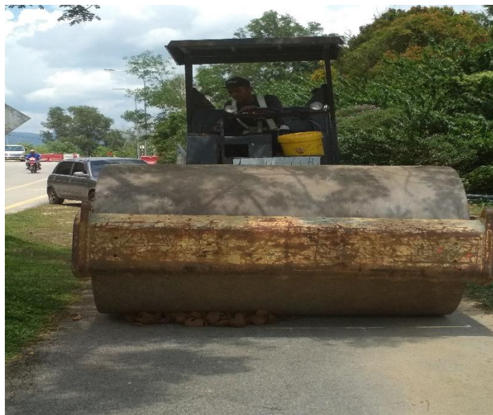
Figure 3.6 Process of crushing coconut shell using roller machine
