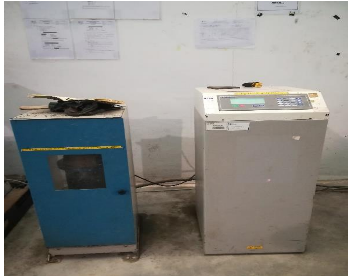
Figure 2.2 Compressive strength test machine
