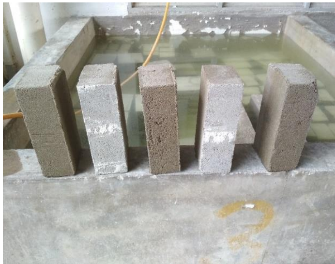
Figure 3.14 Sample of sand brick used for compression test
