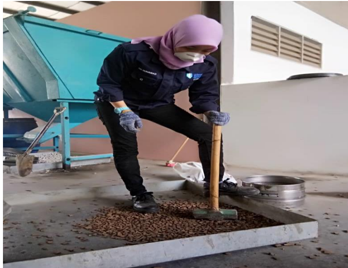
Figure 3.7 Process of crushing coconut shell using hammer
