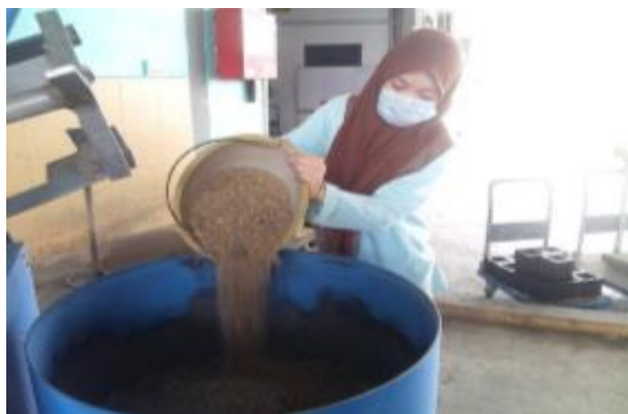
Figure 3.10 Process of mix the materials into mixing machine
