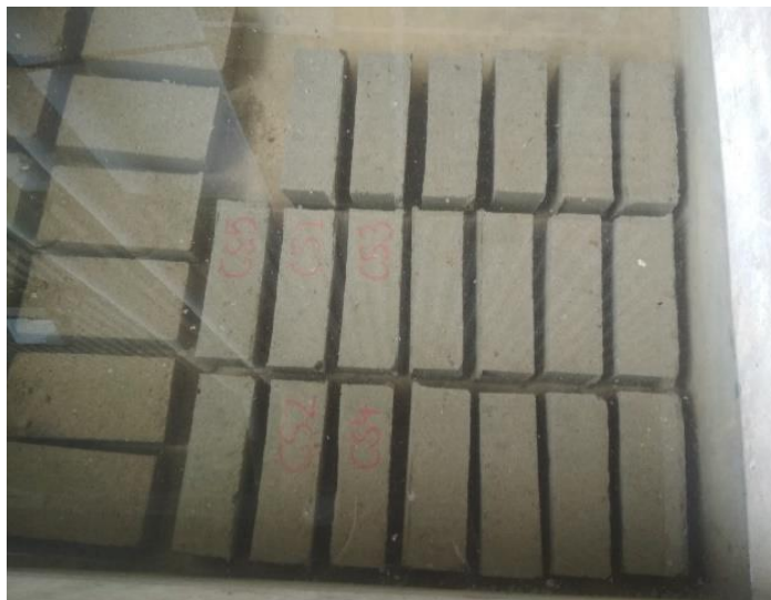
Figure 3.13 Curing process of sand brick
