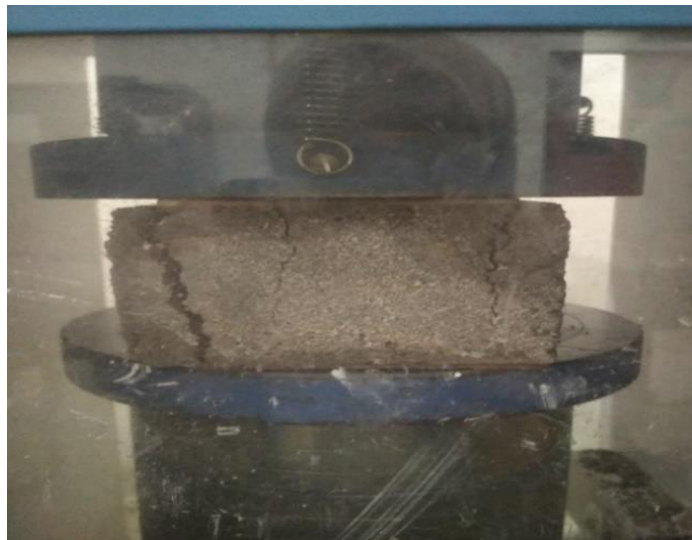
Figure 3.16 Cracked pattern of sand brick
