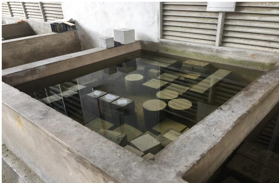
Figure 3.14 Sample was submerged in water for 24 hours after has been dried up in the oven
