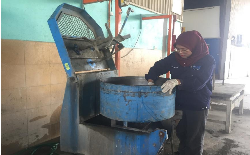
Figure 3.6 The mechanical mixer was use to mix the ingredients
