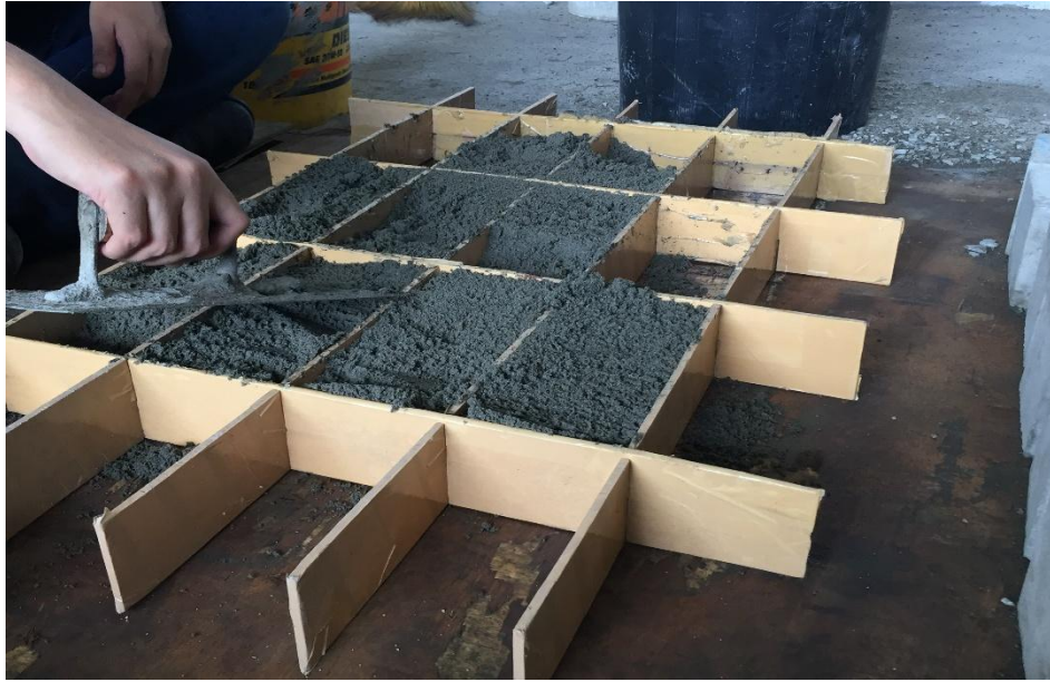
Figure 3.8 Manually compacted by hand
