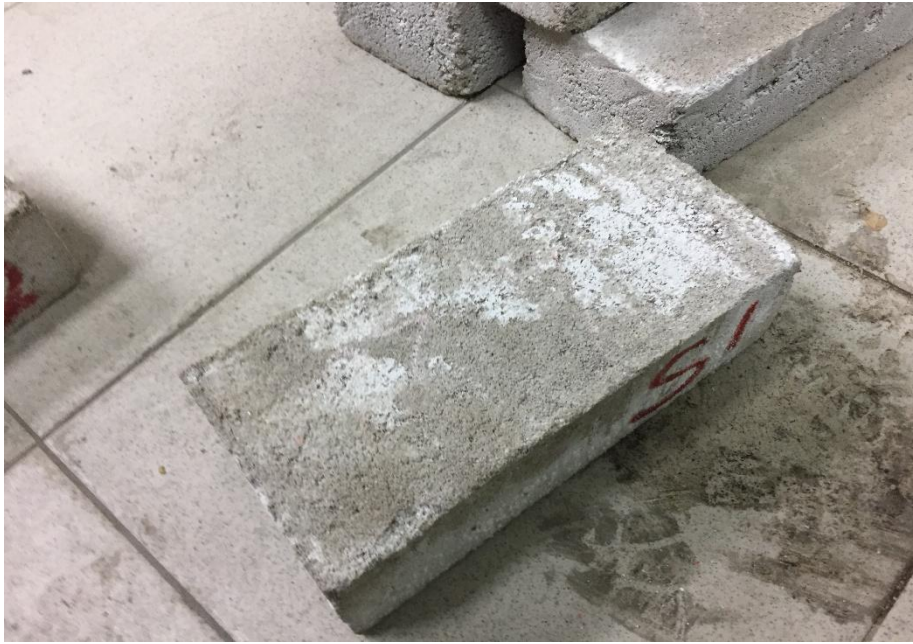
Figure 3.10 All the specimens after demoulded were immersed in water tank until the testing age.
