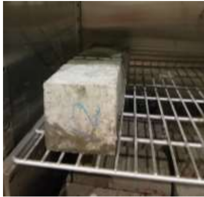
Figure 3.13 The cube placed in oven to oven dry
