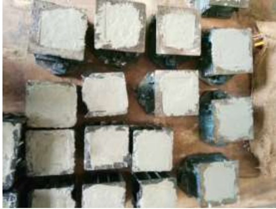
Figure 3.7 The concrete cube in the mold after casting
