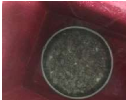
Figure 3.11 The aggregates immersed in the water for 24 hours
