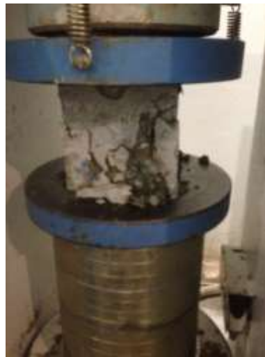
Figure 3.12 The specimen tested by compression machine testing
