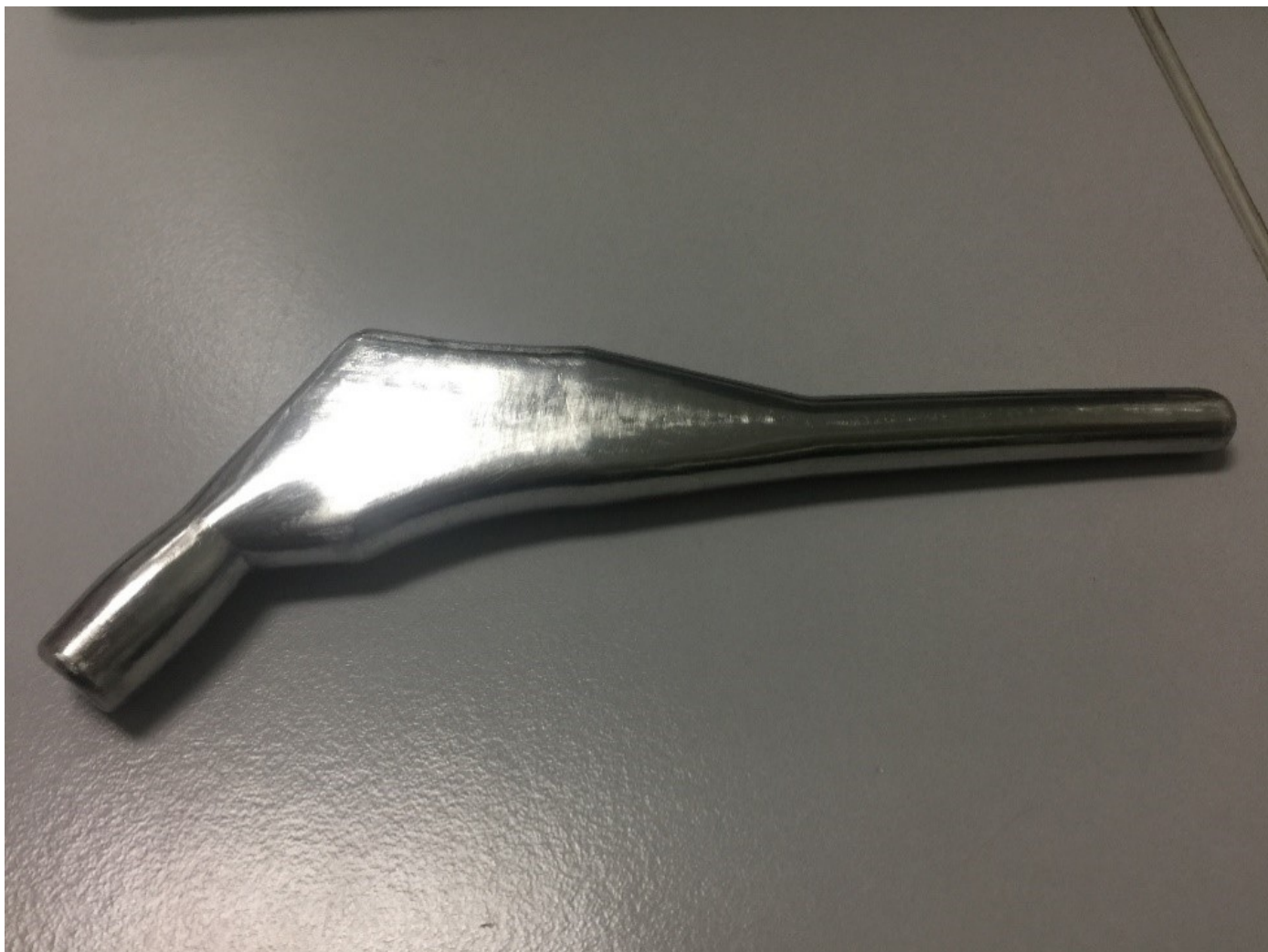
Figure 2: Successful printed hip femoral implant
