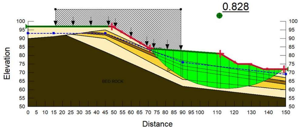
**Figure 2.** Back analysis results with critical FOS.
