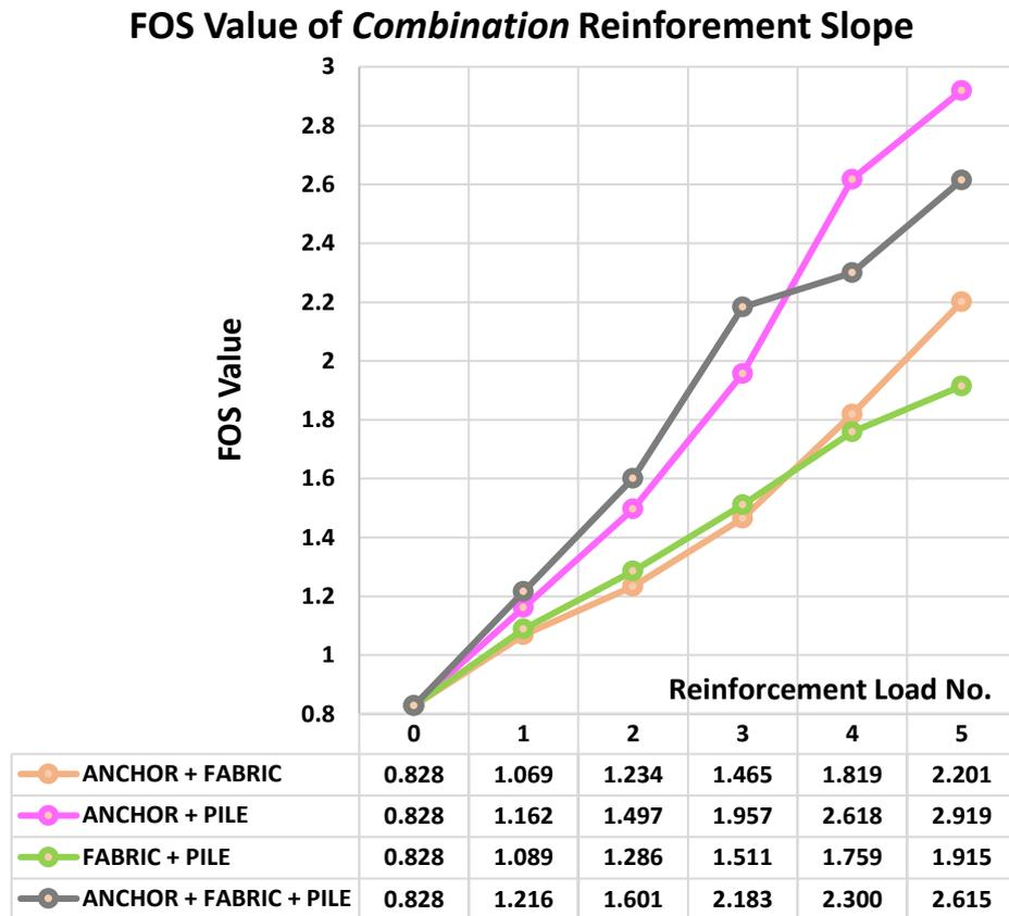
**Figure 4.** Design analysis results of combination reinforcement slope.
