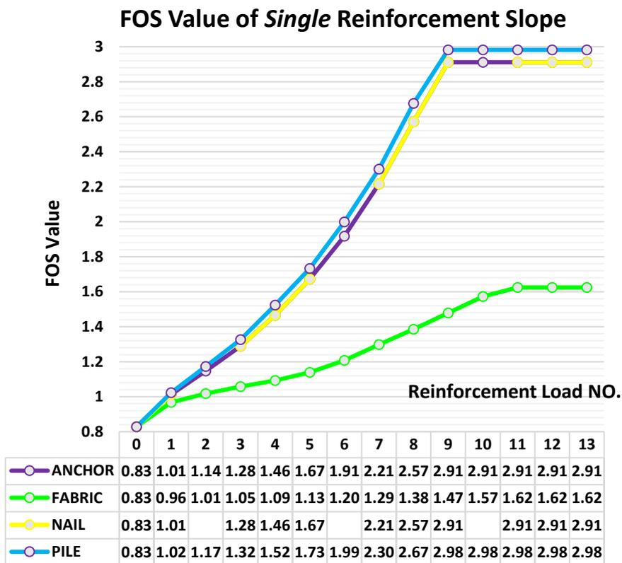
**Figure 3.** Design analysis results of single reinforcement slope.
