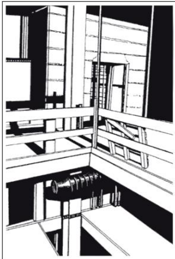
Figure 4.11 Edge Protection; Guard-rails and Toe Boards
