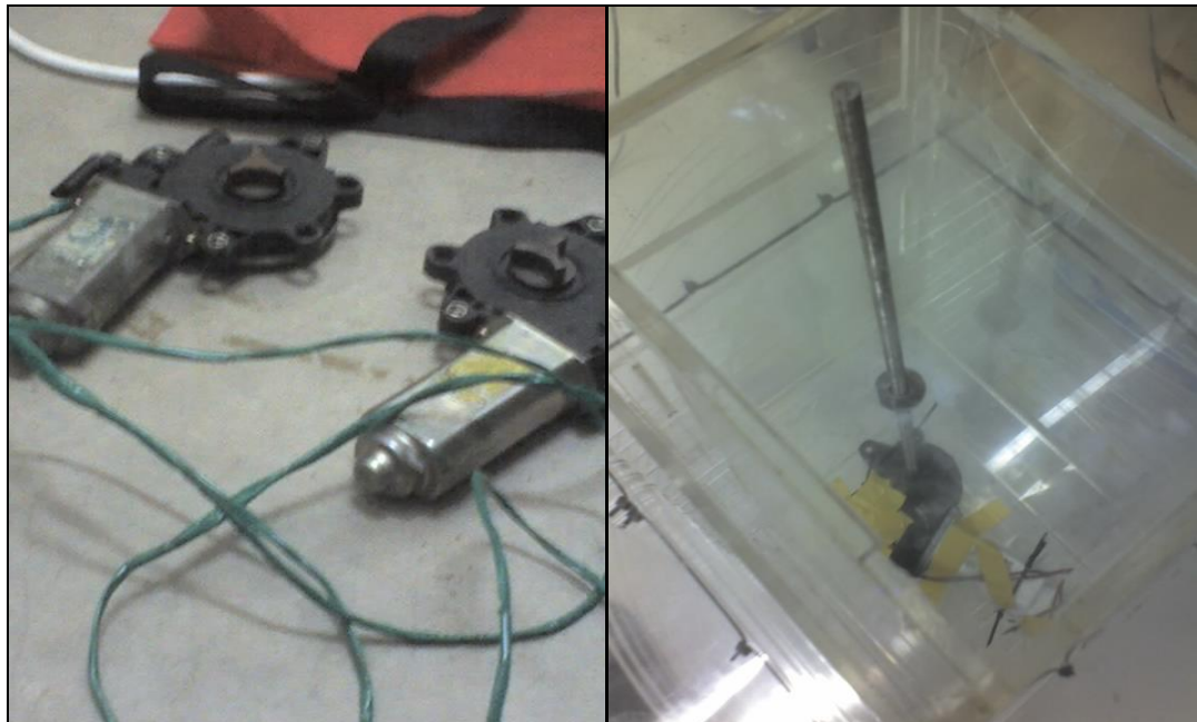
Figure 4.3 Power window motor (left) and motor connected to rostrum using the lead screw (right)
