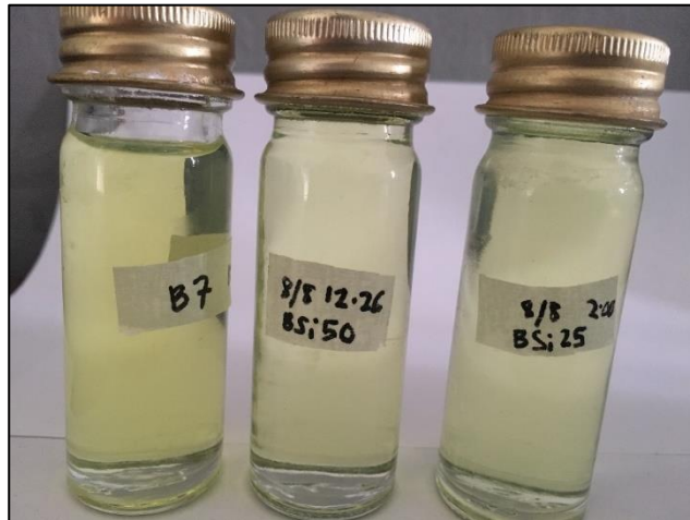
Figure 3. SiO 2 nanoparticle-biodiesel fuel blends after preparation.
