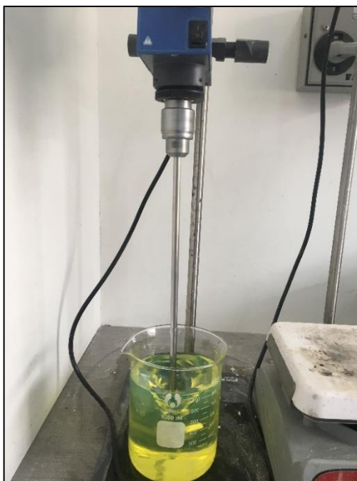
Figure 1. Homogenizer mixer used for biodiesel and SiO 2 nano particles blend.
