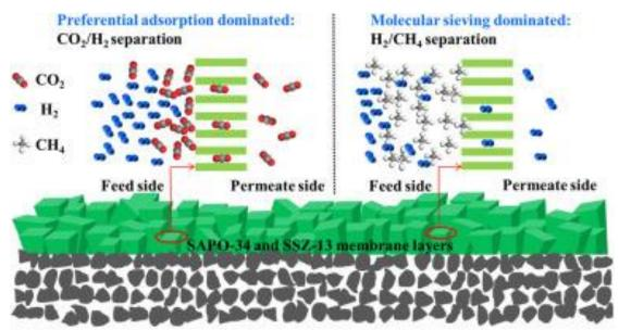
Fig. 2. High-flux CHA zeolite membranes for H<sub>2</sub> separations [43]
