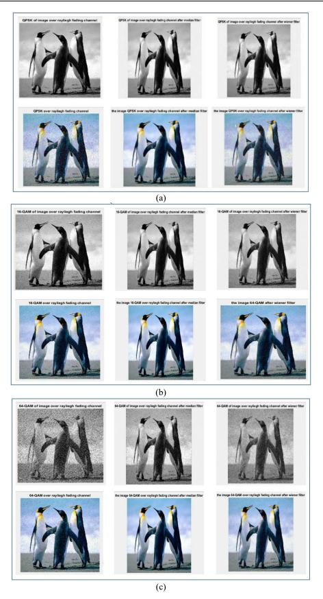
Figure 3. Comparison of recovered images at the system receiver without filter, with median filter and with wiener filter for different modulation schemes over Rayleigh fading channel;(a) QPSK modulation sheme, (b) 16-QAM modulation scheme, and (c) 64-QAM modulation sheme
