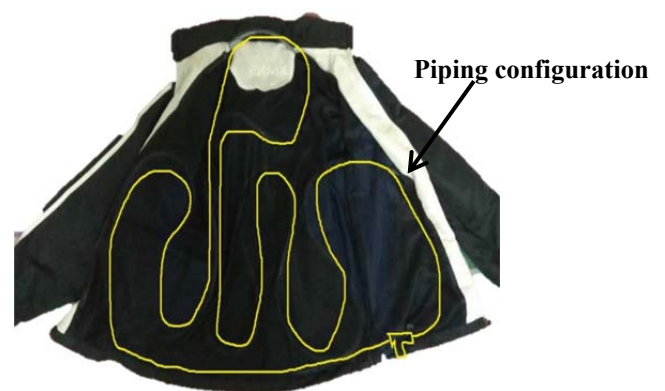
Figure 4. Piping configuration of the cooling jacket
