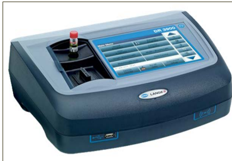
Figure 3.3 DR3900 portable spectrophotometer
