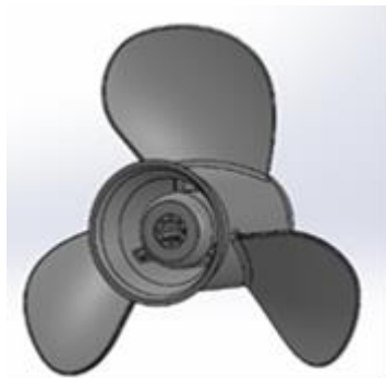
Figure 1. CAD model of three blades propeller structure.
