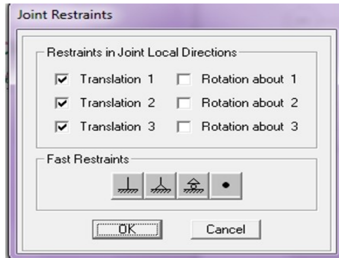
Step 3.14 Add restraint at the base condition
