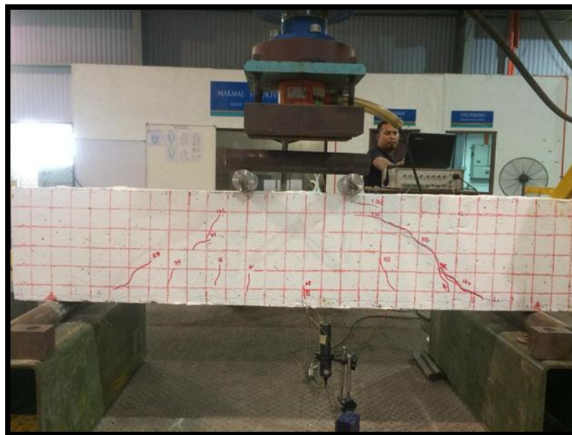
Figure 4.3: Flexural Failure for Controlled Beam
