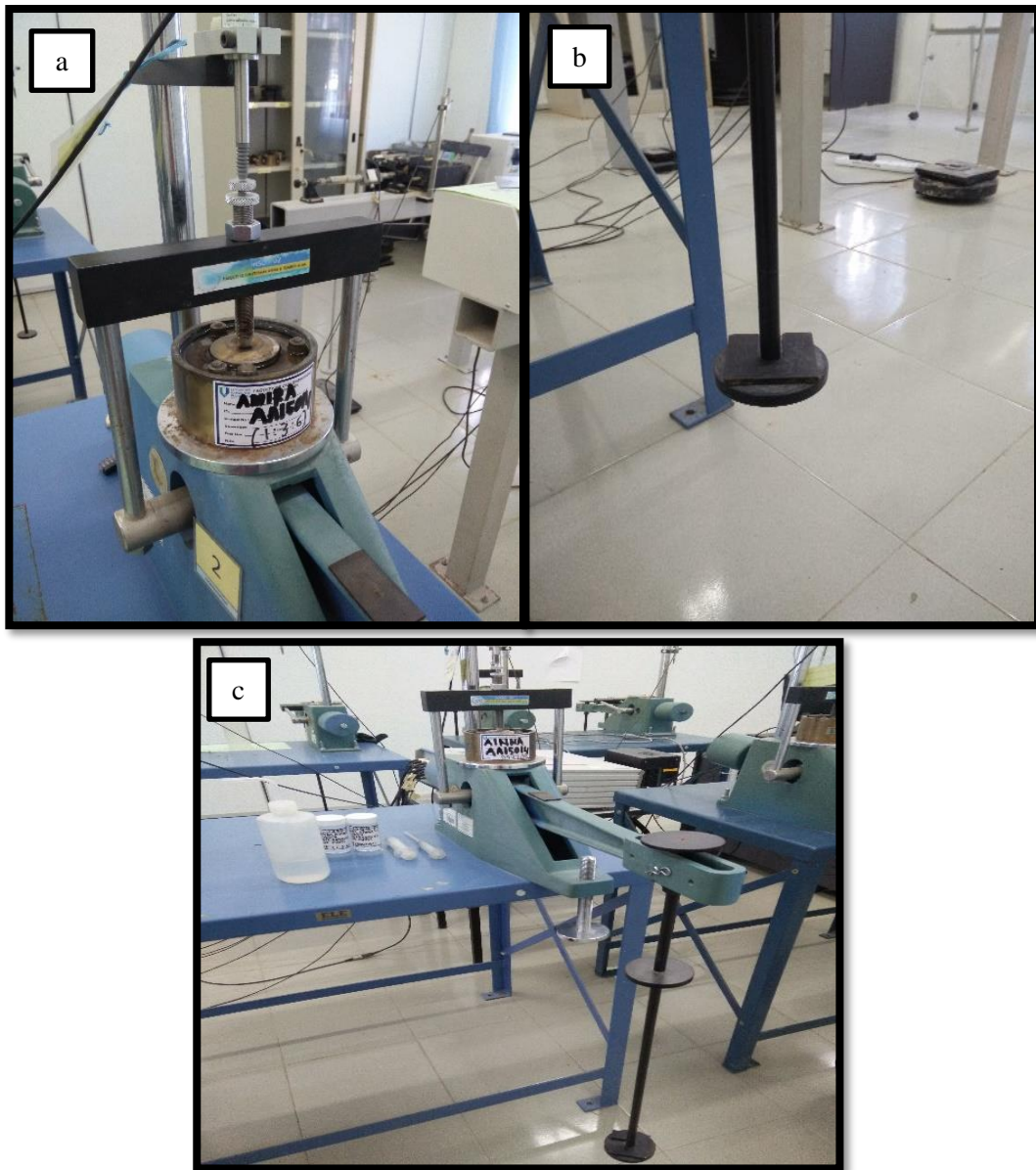
Figure 3.9 Set-up apparatus of soil sample in the ring a) placed the ring at the top of oedometer apparatus b) applied load pressure c) overview of oedometer set-up apparatus
