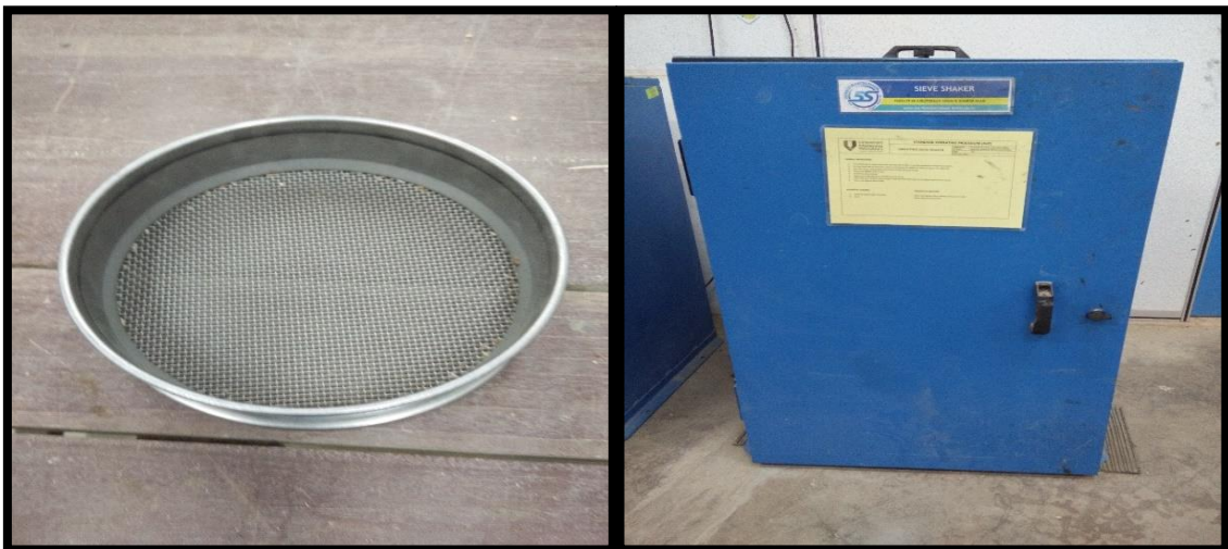
Figure 3.1 Soil samples were sieved passing sieve no 425 \mu m using sieve shaker
