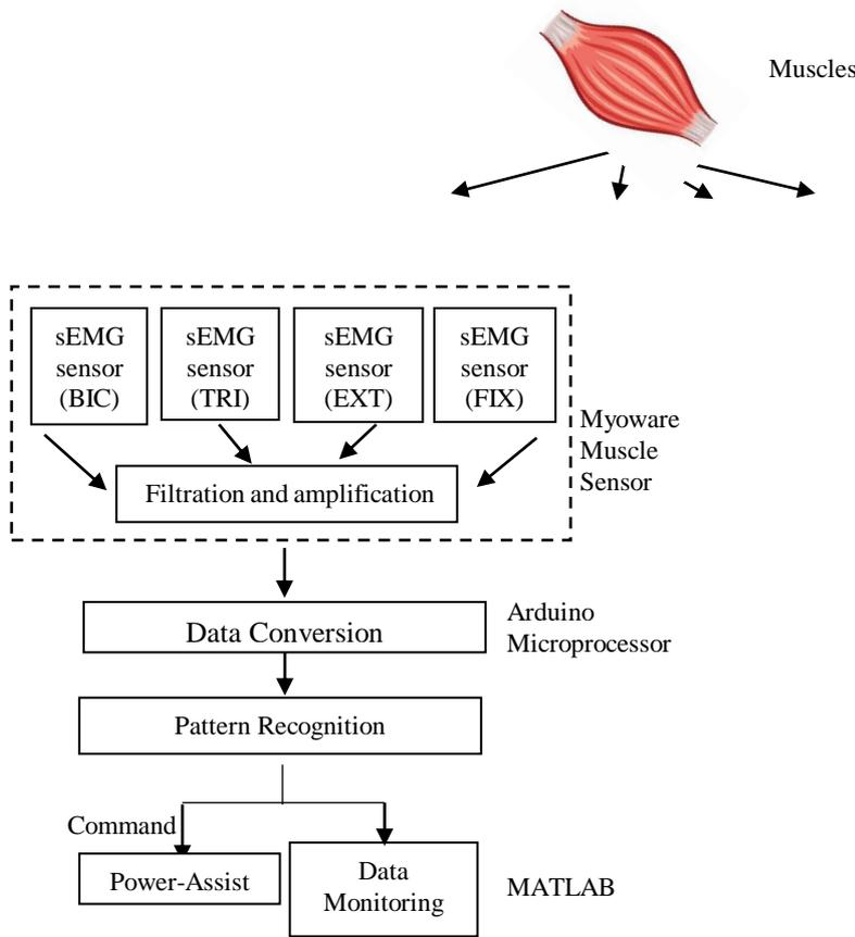
Figure 5: sEMG Data Acquisition for Validation Test
