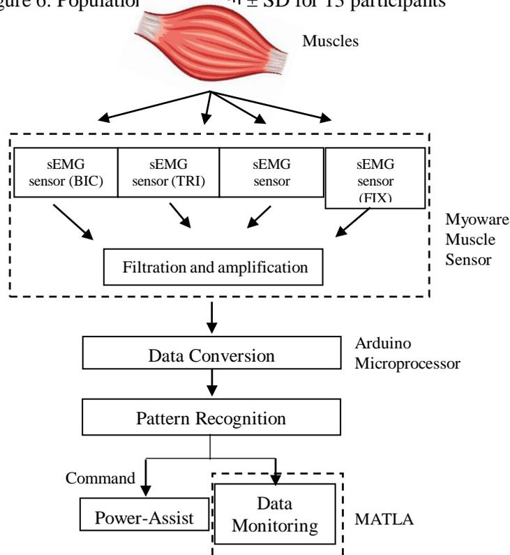
Figure 6: sEMG Data Acquisition for Validation Test
