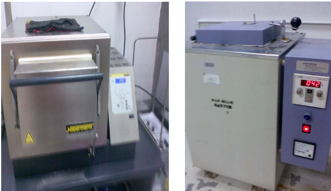
Figure 3.5: Box furnace used to perform annealing and recovery process
