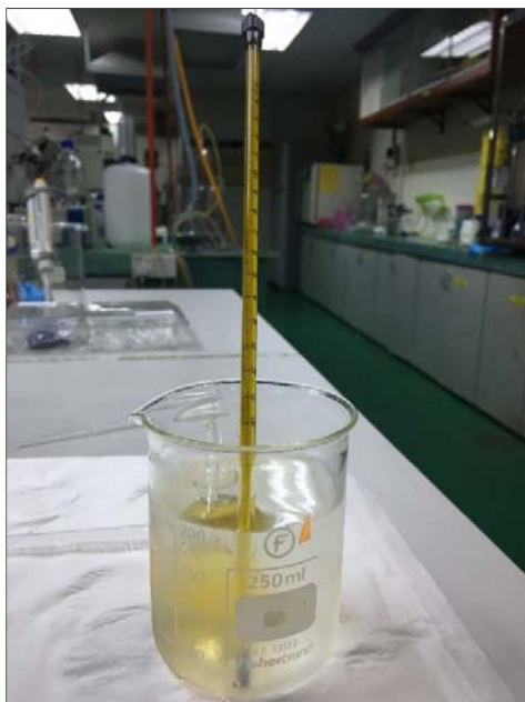
Figure 7. Nanoparticle-diesel blends ASTM D1298.
