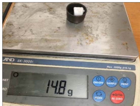
Figure 10 (c). Mass of Bucket + sample measured by electronic weighing scale.
