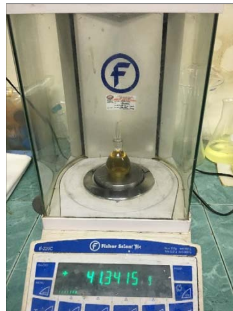
Figure 8. Mass of pycnometer and nanoparticles-diesel blends.
