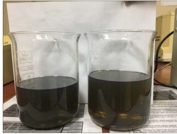
Figure 3. Left: before mixing by ultrasonic, right: after mixing by ultrasonic.
