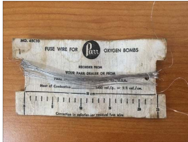
Figure 10 (a). Fuse wire.
