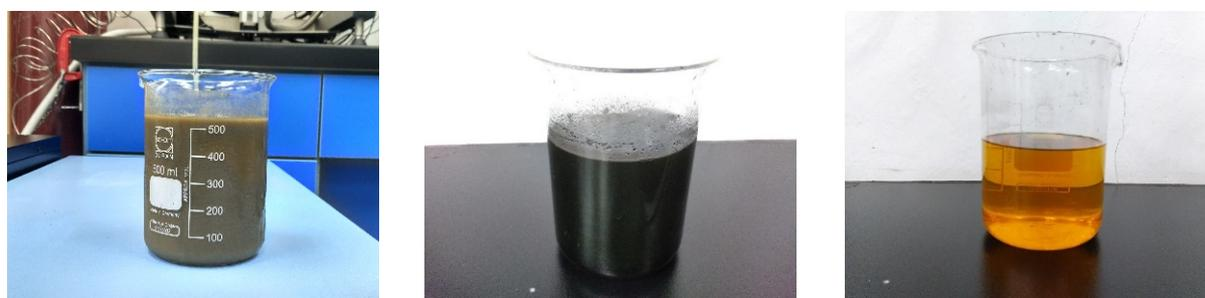
**Figure 2.** (from left) Fresh POME, liquid product of NOHT at 533 K & 8 h and liquid product of OHT at 533 K & 8 h.
