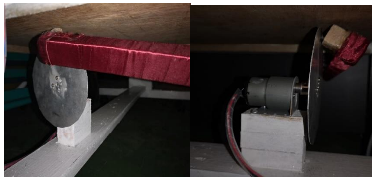
Figure 4.14 Rotating mechanism of the baby cradle
