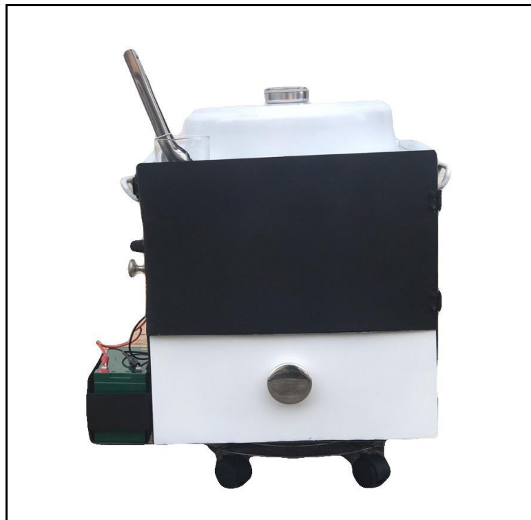
Figure 1.2: The Charcoal Barbeque with Air Ventilation System
