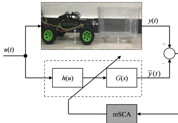
**Figure 5.** Block diagram of Hammerstein model based mSCA
