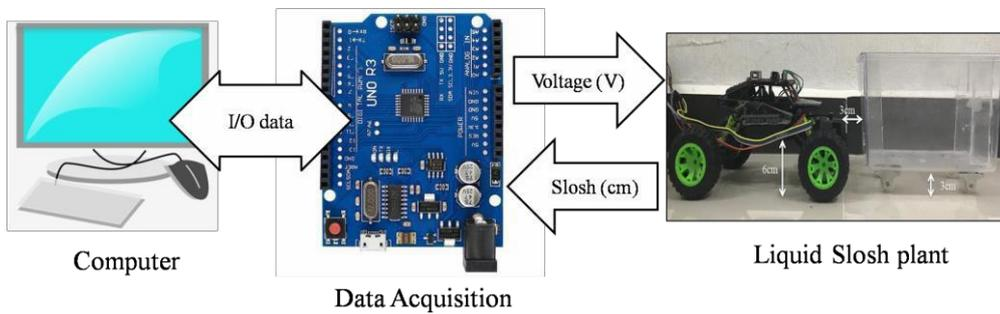
**Figure 2.** Schematic diagram of liquid slosh experimental rig
