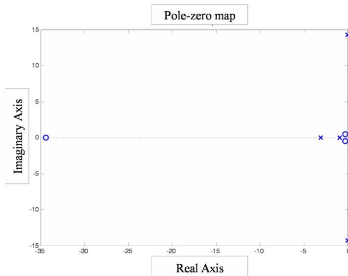
**Figure 8.** Pole-zero map of transfer function  $G(s)$
